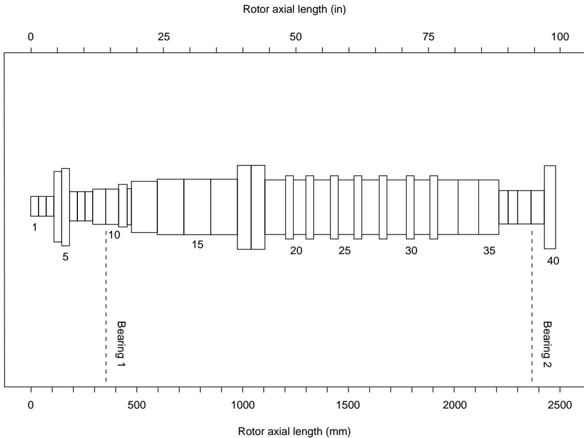
Figure 1-17—Rotor Model Cross Section of an Eight-Stage 12 MW (16,000 HP) Steam Turbine
