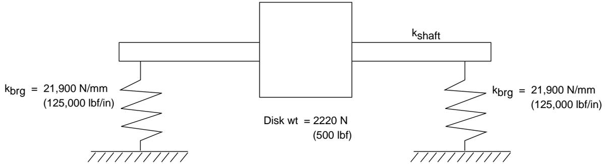
**A SIMPLIFIED MODEL OF A BEAM-TYPE ROTATING MACHINE**
