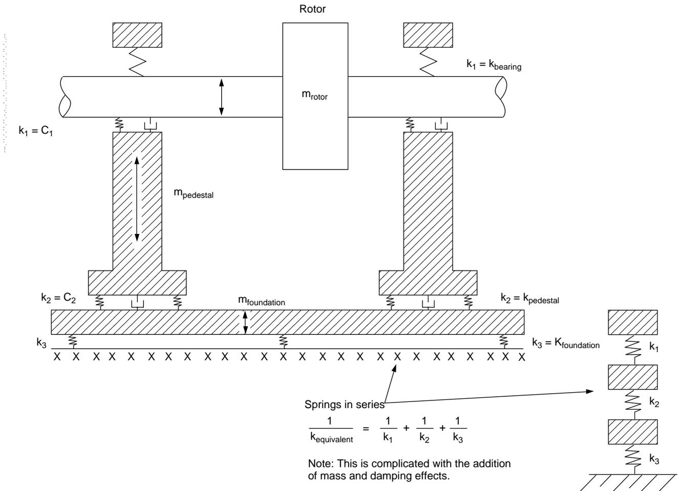
Figure 1-47—Schematic of a Rotor With Flexible Supports and Foundation
