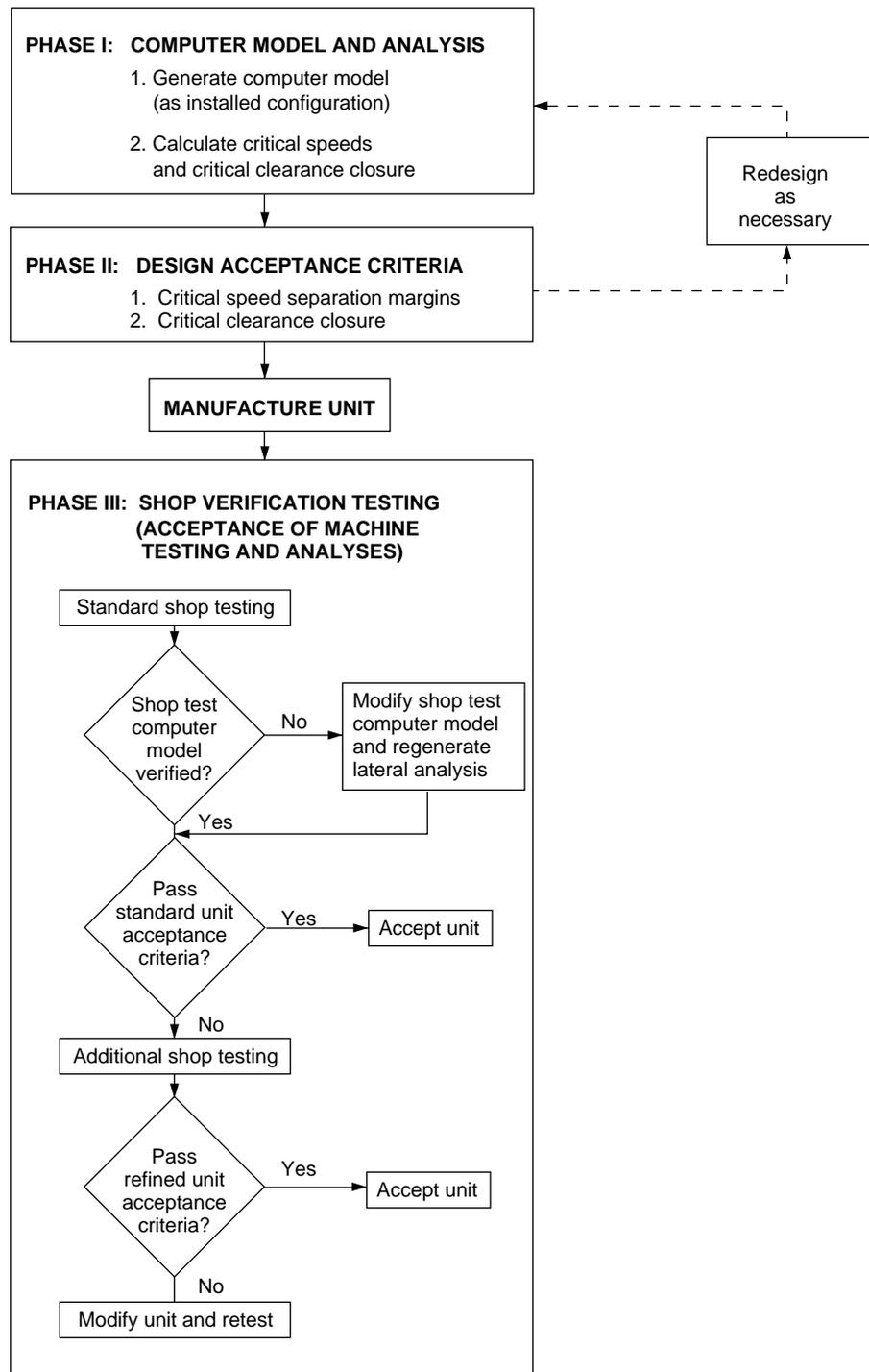
Figure 1-33—Three-Phase Vibration Acceptance Program
