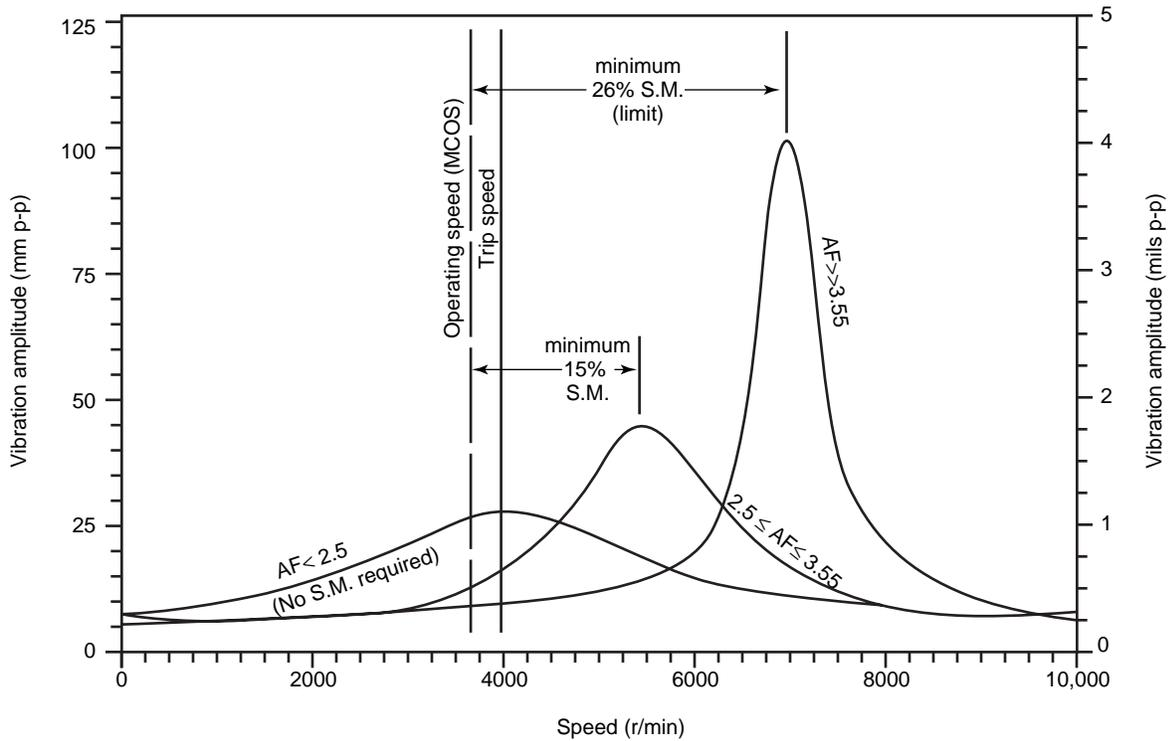
Figure 1-50—API Required Separation Margins for Operation Below a Critical Speed
