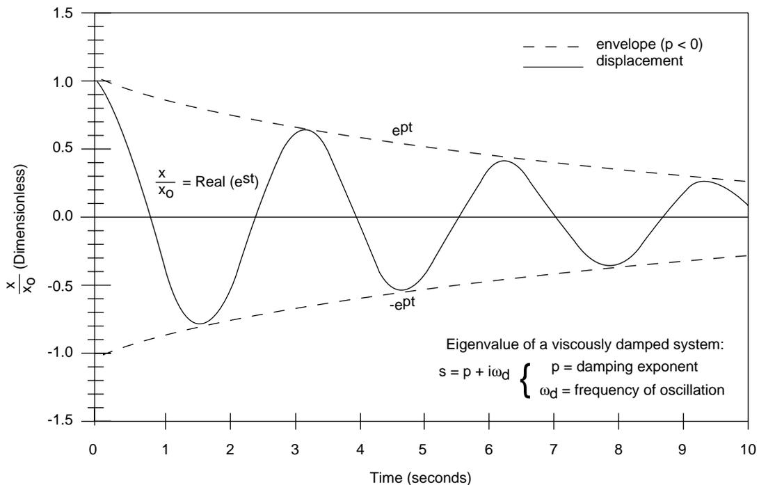
Figure 1-12—Motion of a Stable System Undergoing Free Oscillations
