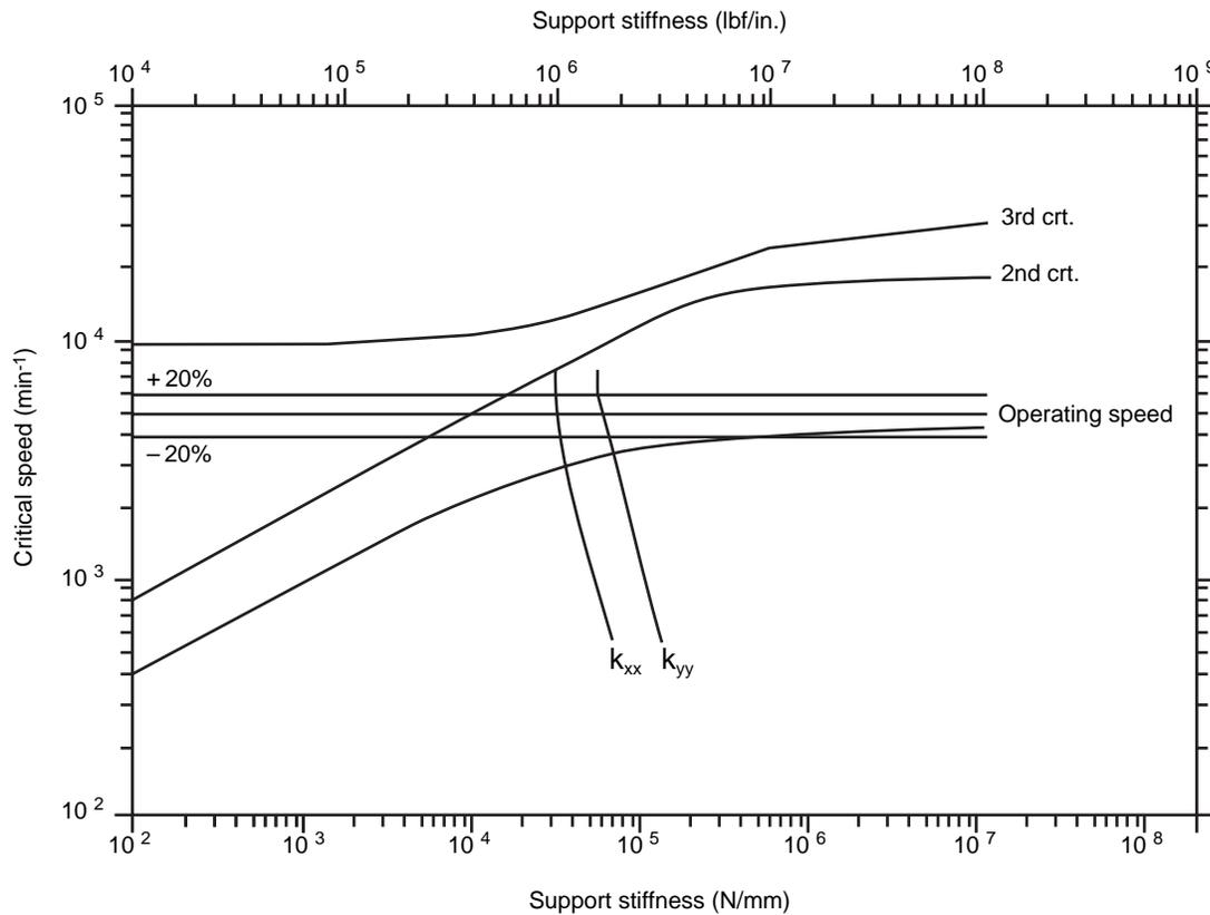
Figure 1-46—Undamped Critical Speed Map for an Eight-Stage 12 MW (16,000 HP) Steam Turbine
