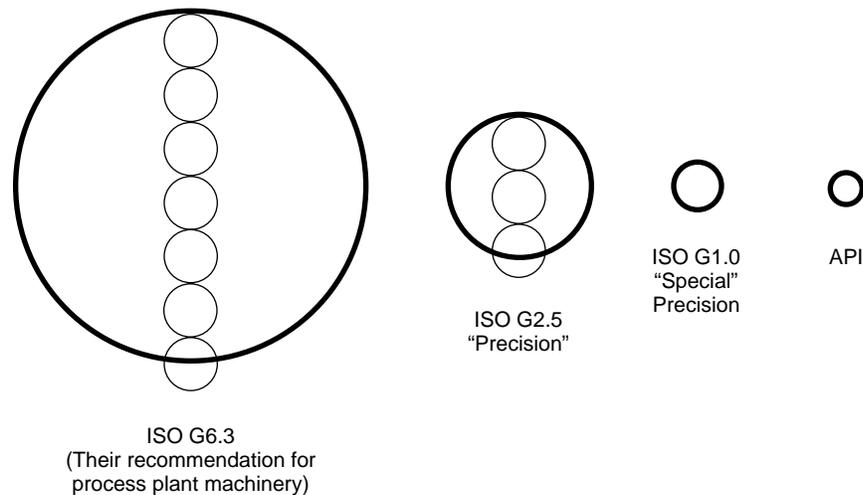
Figure 3-3—Shaft Centerline Unbalance Orbits
