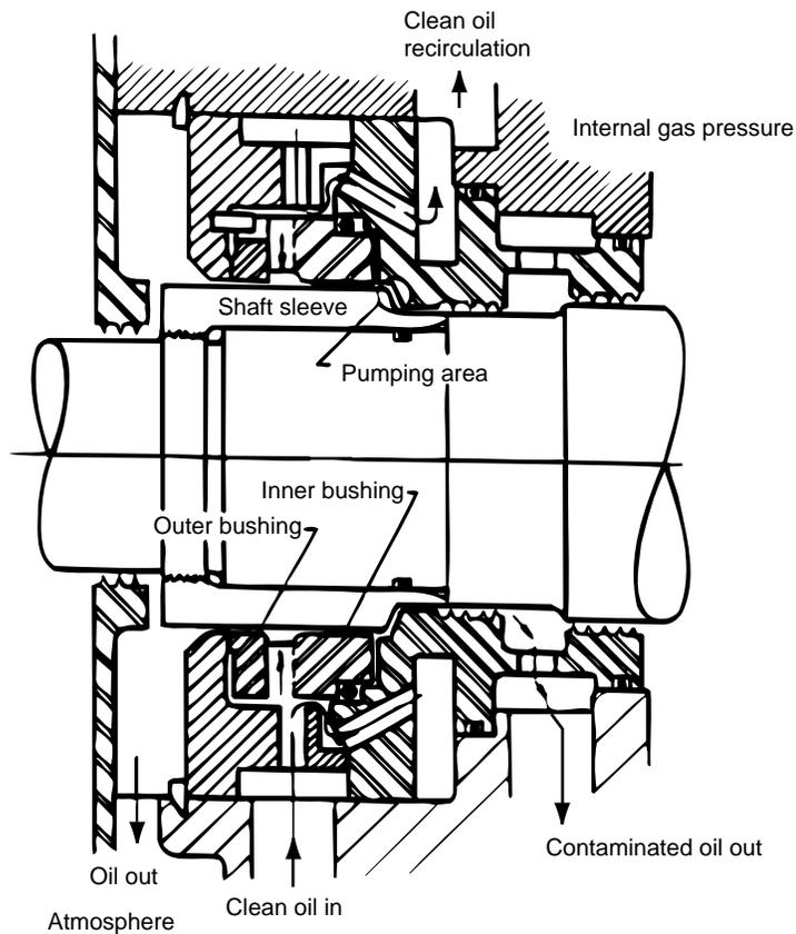
Figure 1-31—Liquid-Film Shaft Seal with Pumping Bushing
