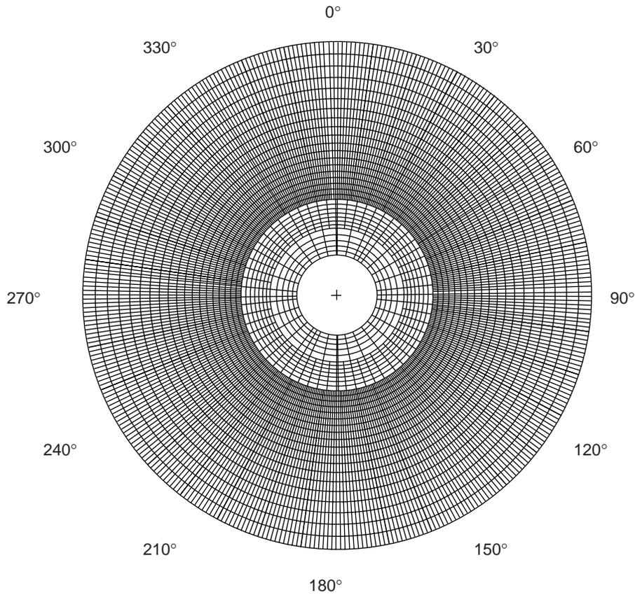
The circle you have drawn must contain the origin of the polar chart. If it doesn't, the residual unbalance of the rotor exceeds the applied test unbalance.
