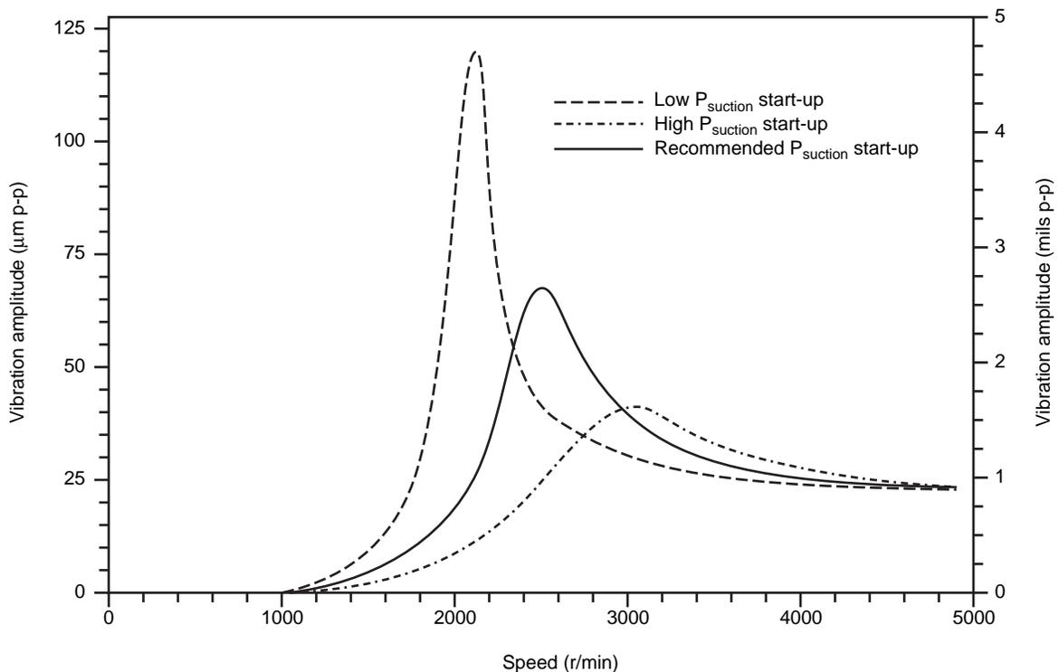
Figure 1-26—Midspan Rotor Unbalance Response of a High Pressure Centrifugal Compressor for Different Suction Pressures on Startup
