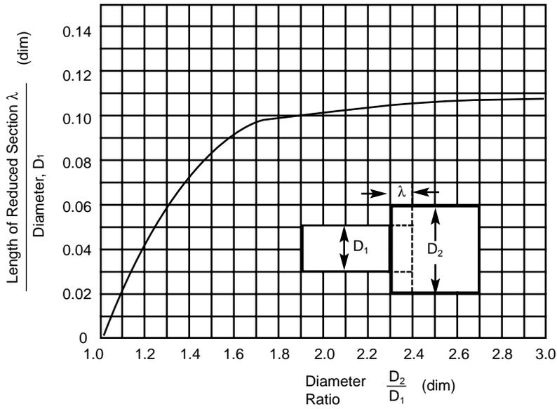
Figure 2-10—Effective Penetration of Smaller Diameter Shaft Section Into A Larger Diameter Shaft Section Due To Local Flexibility Effects (Torsion only)
