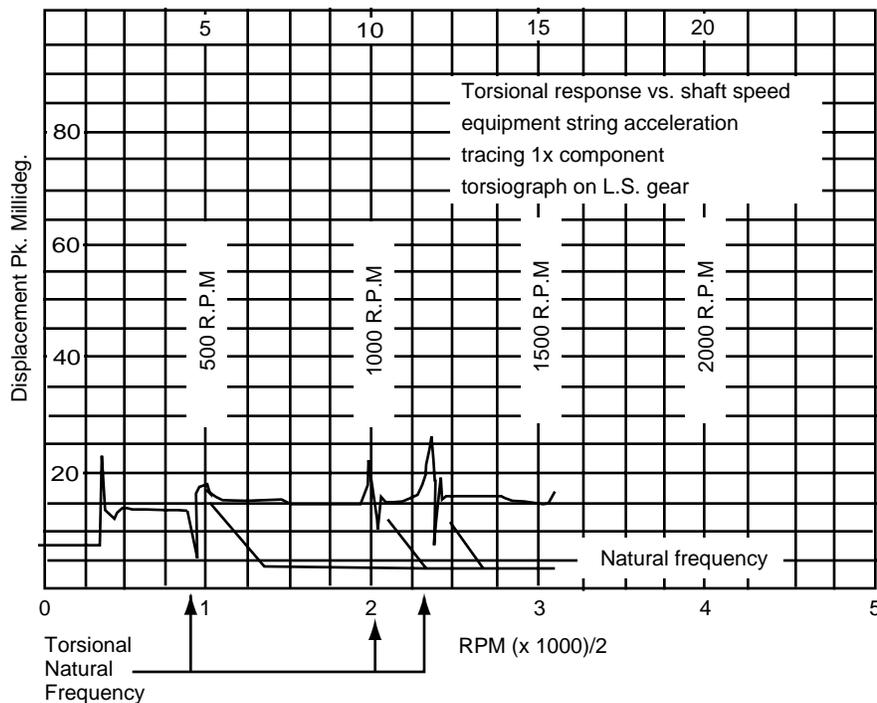
Figure 2-30—Sample Torsiograph Measurements
