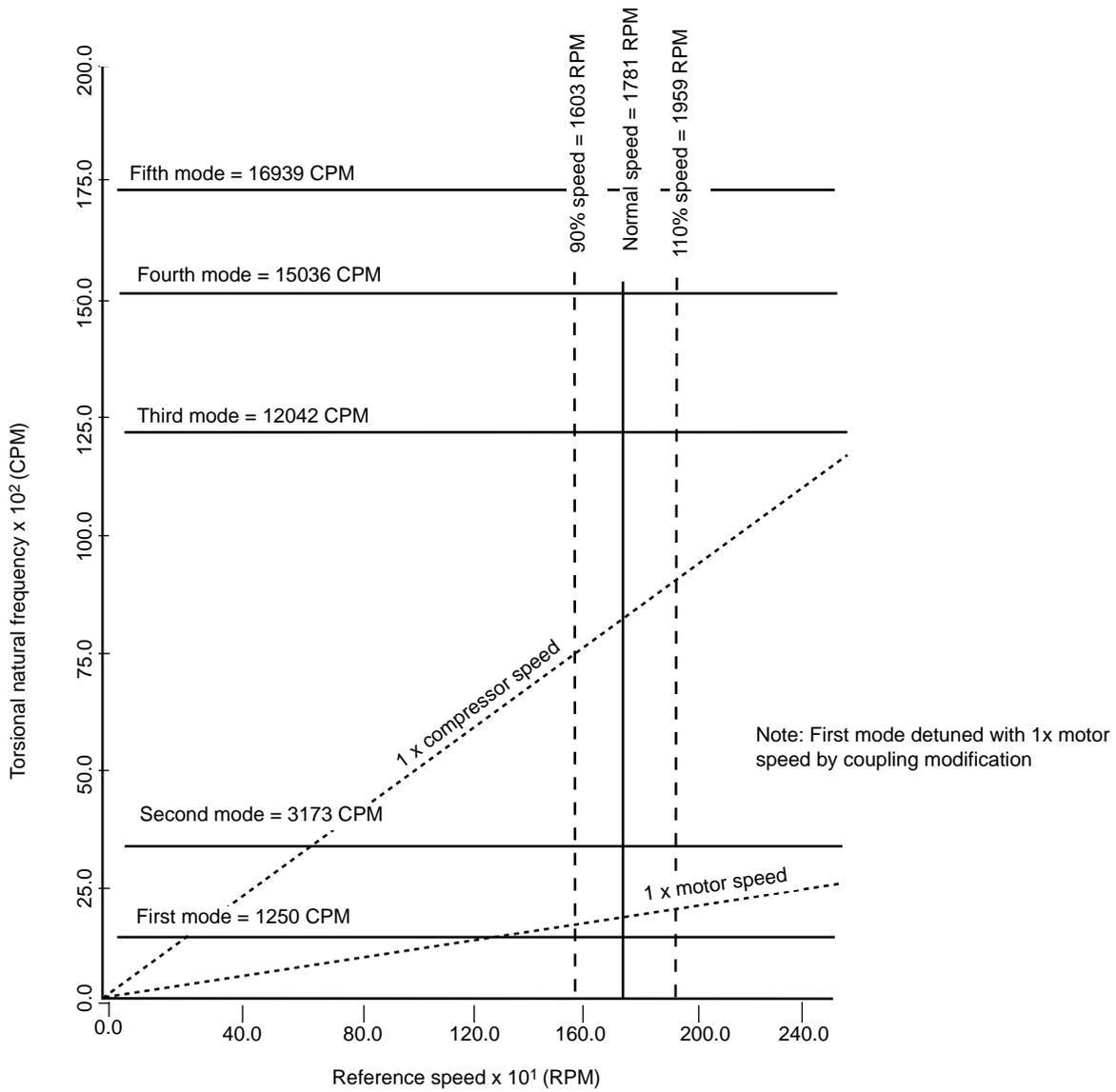
Figure 2-21—Sample Train Torsional Campbell Diagram for a Typical Motor-Gear-Compressor Train (With Acceptable Torsional Natural Frequency Separation Margins)
