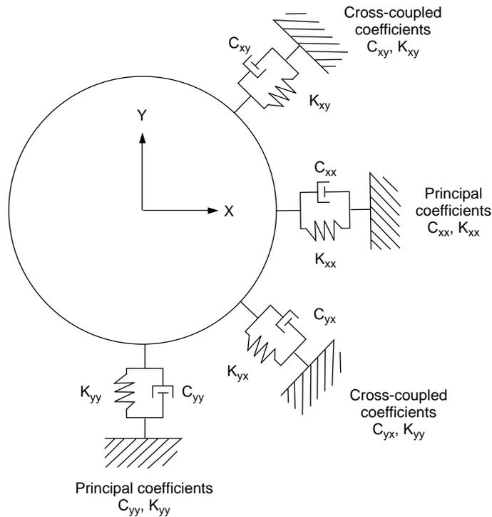
Figure 1-20—Linear Bearing Model Used in Most Rotor Dynamics Analysis
