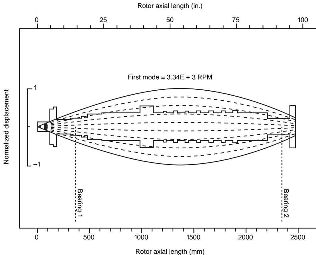
Figure 1-35—First Mode Shape for Eight-Stage Steam Turbine
