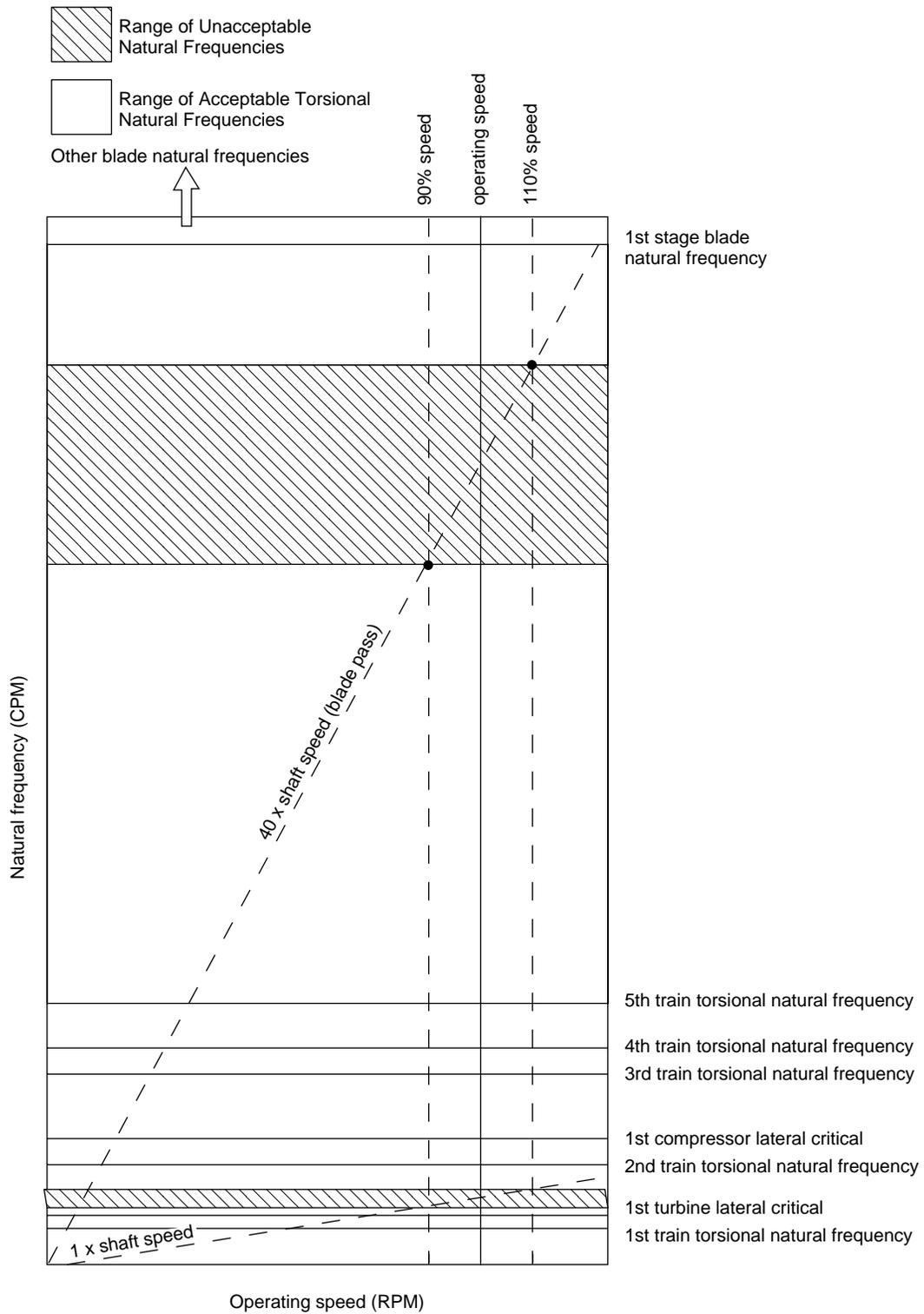
Figure 1-4—Sample Train Campbell Diagram for a Typical Turbine-Compressor Train
