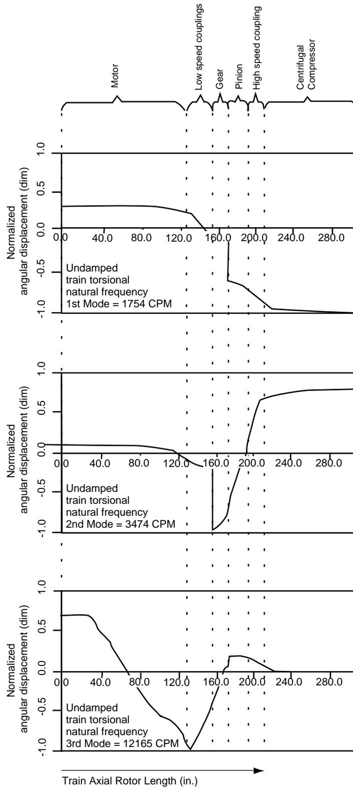
Figure 2-19—Torsional Modeshapes for a Typical Motor-Gear-Compressor Train
