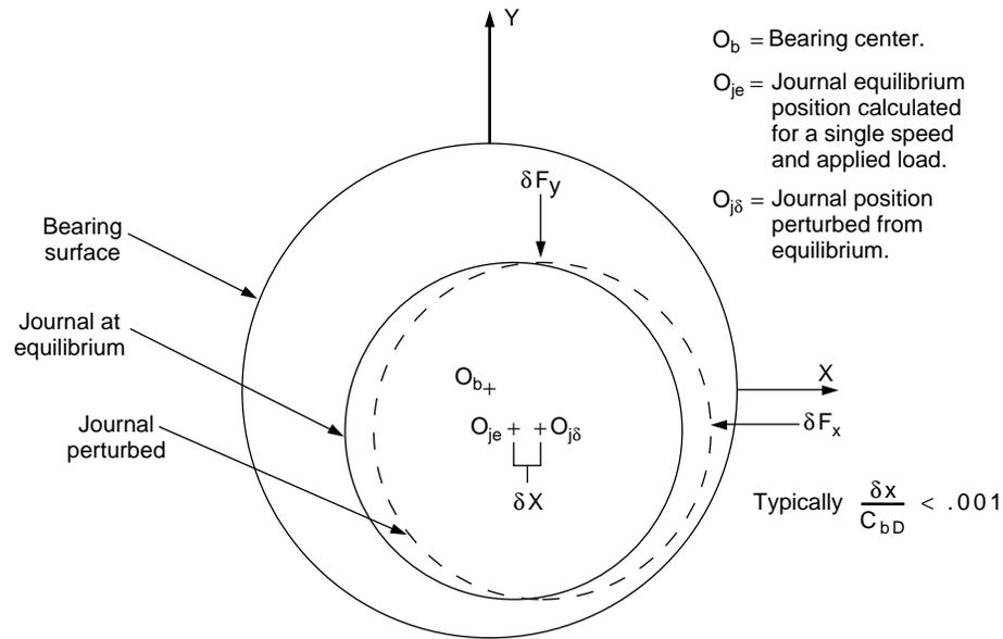
Note: The figure above displays how two of the four bearing stiffness coefficients  $K_{xx}$  and  $K_{yx}$  are calculated as shown below:
