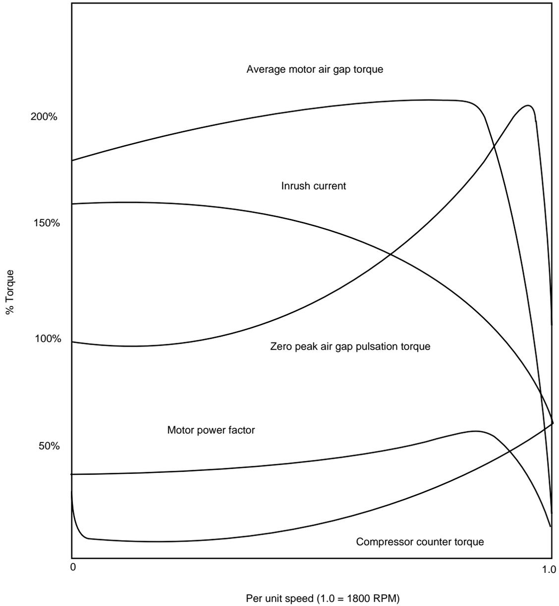
Figure 2-28—Speed-Torque Characteristics of a Solid Synchronous Pole Motor
