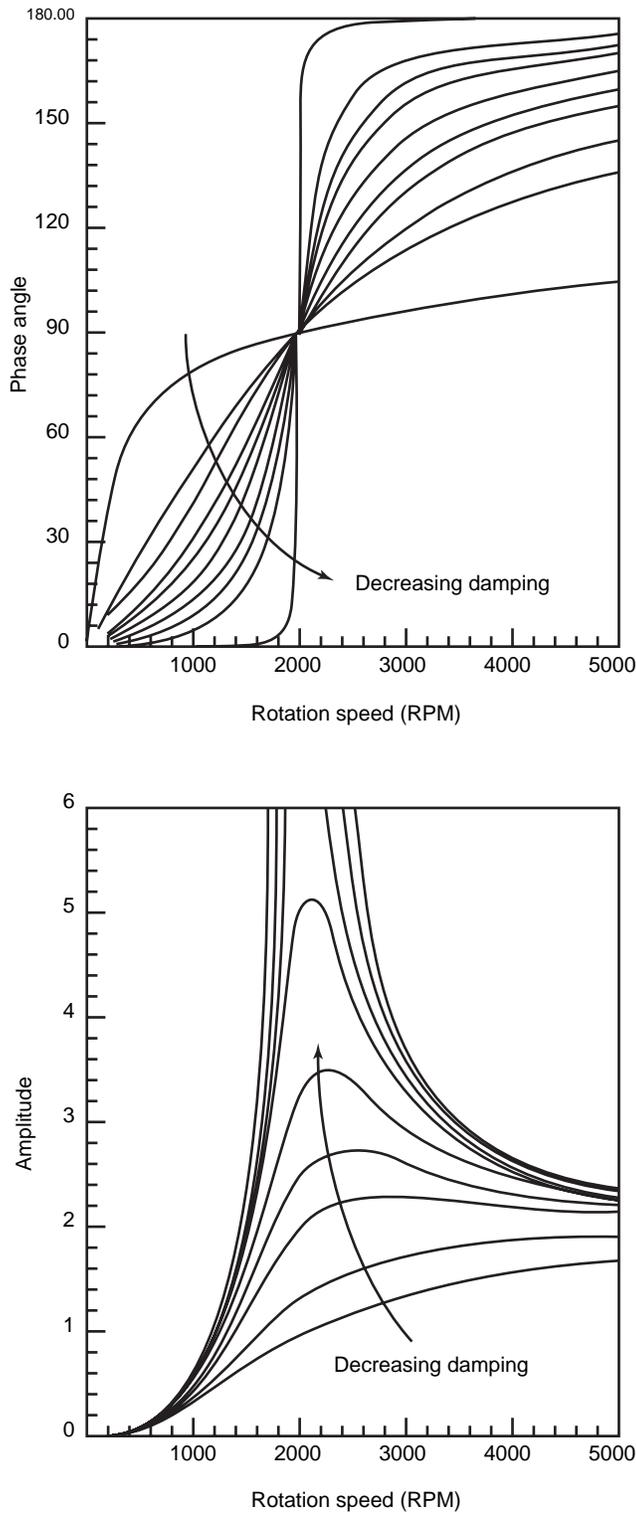
Figure 1-11—Effect of System Damping on Phase Angle and Response Amplitude
