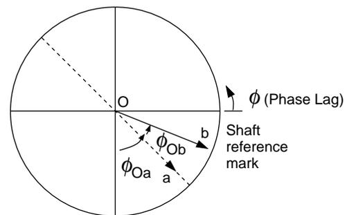
Step 3. Generate response and unbalance vector triangles and then calculate the residual unbalance vector,  $U_{\text{residual}}$ . Note that the two triangles displayed in these diagrams are assumed to be geometrically similar.
