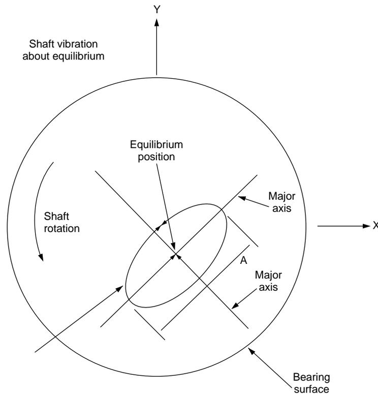
Figure 1-54—Elliptical Orbit of Shaft Vibration Showing Major and Minor Axes of Lissajous Pattern
