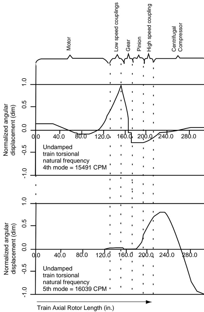
Figure 2-19—Torsional Modeshapes for a Typical Motor-Gear-Compressor Train (Continued)
