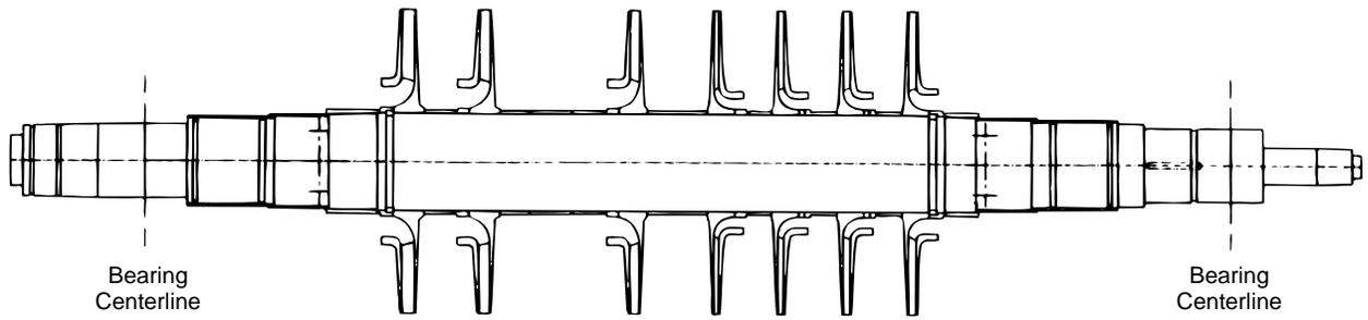
Figure 1-25—Seven Stage High Pressure Natural Gas Centrifugal Compressor
