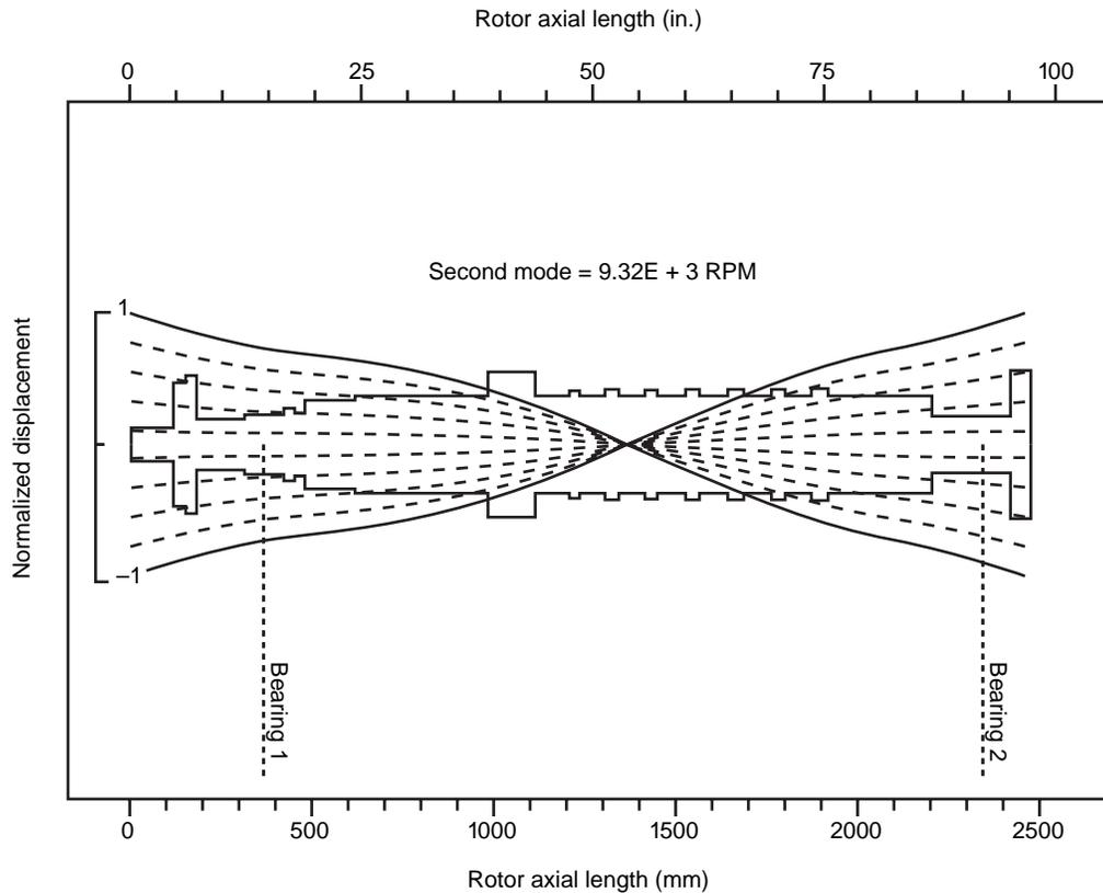
Figure 1-36—Second Mode Shape for Eight-Stage Steam Turbine (Generated by Undamped Critical Speed Analysis)
