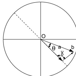
Figure 1-52—Calculating the Test Unbalance
