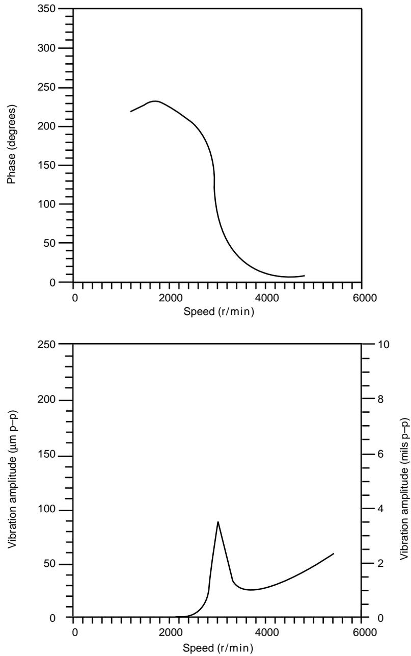
Figure 1-53—Bode Plot For First Mode Test Unbalance
