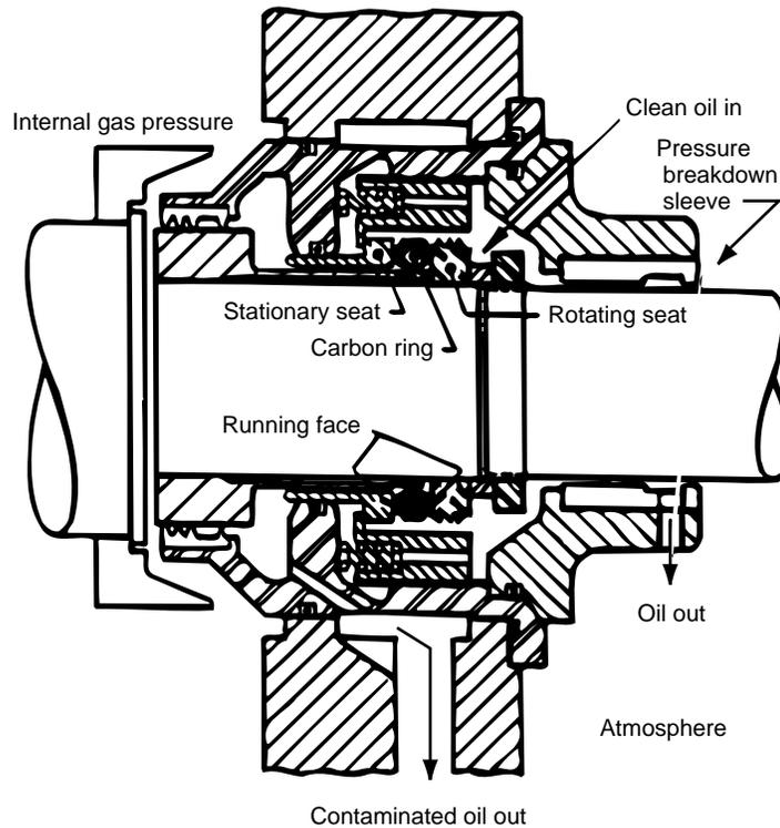
Figure 1-28—Mechanical (Contact) Shaft Seal
