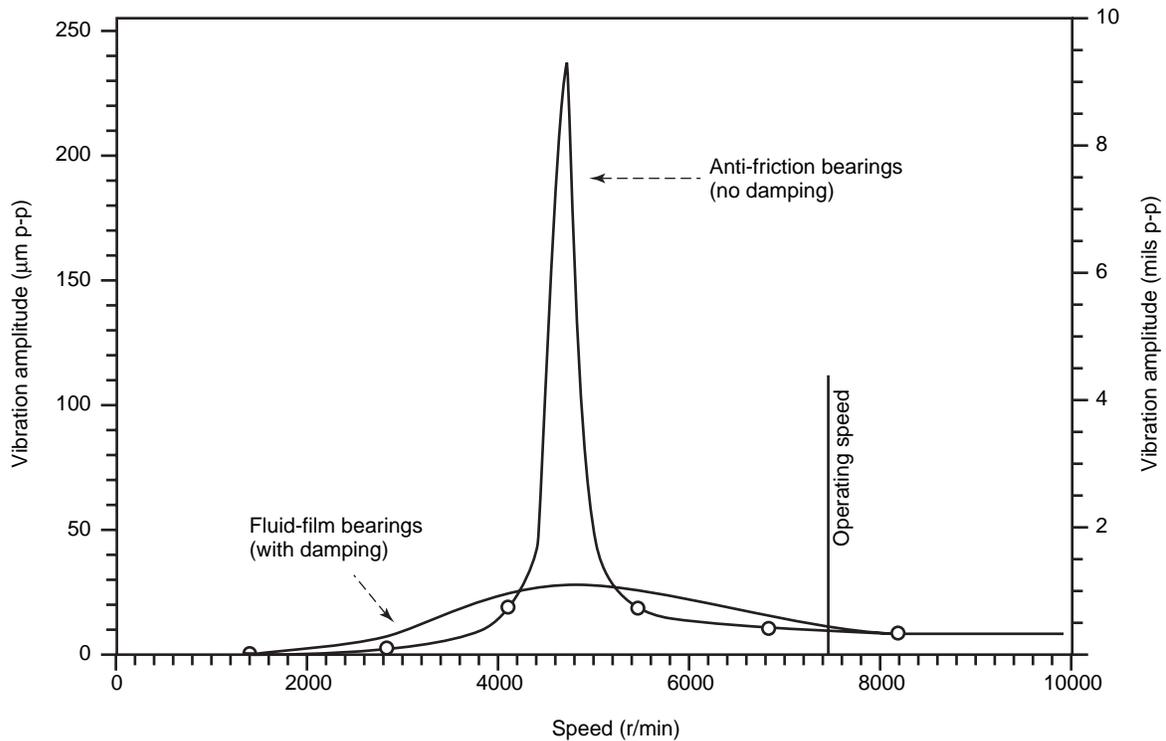
Figure 1-40—Comparison of First Mode Response With Fluid-Film Bearings and Anti-Friction Bearings
