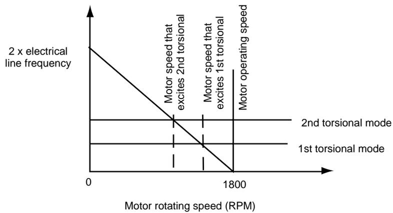
Figure 2-27—Frequency of Synchronous Motor Pulsating Torque (4 Pole Synchronous Motor)
