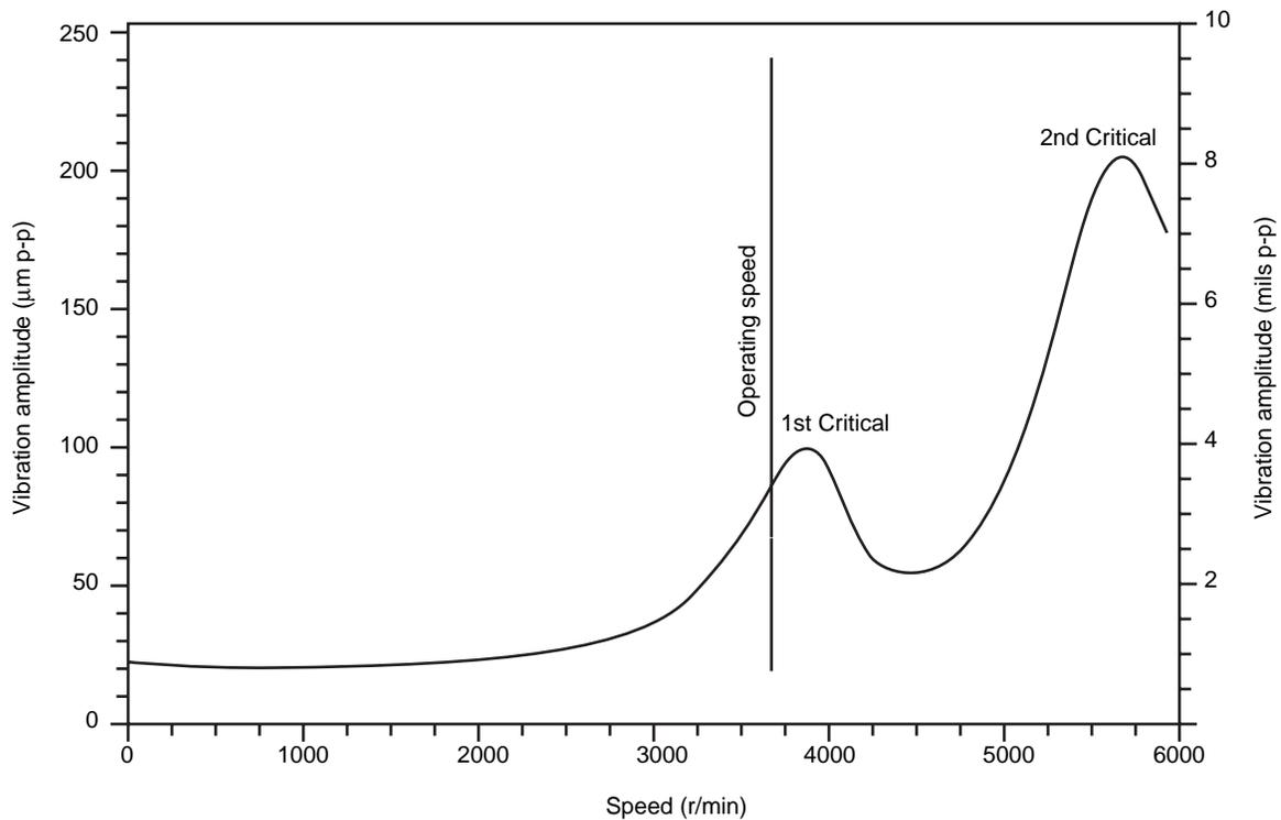
Figure 1-42—Response of a Constant Speed, Two-Pole Motor
