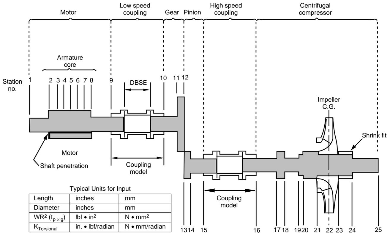
Note: Coupling vendors typically provide  $WR^2$  and  $K_{Torsional}$  for each coupling. The  $WR^2$  value does not include the  $WR^2$  of the coupling journal (shaft inside the coupling HUB). The  $K_{Torsional}$  value typically assumes  $1/3$  shaft penetration into the coupling HUB.
