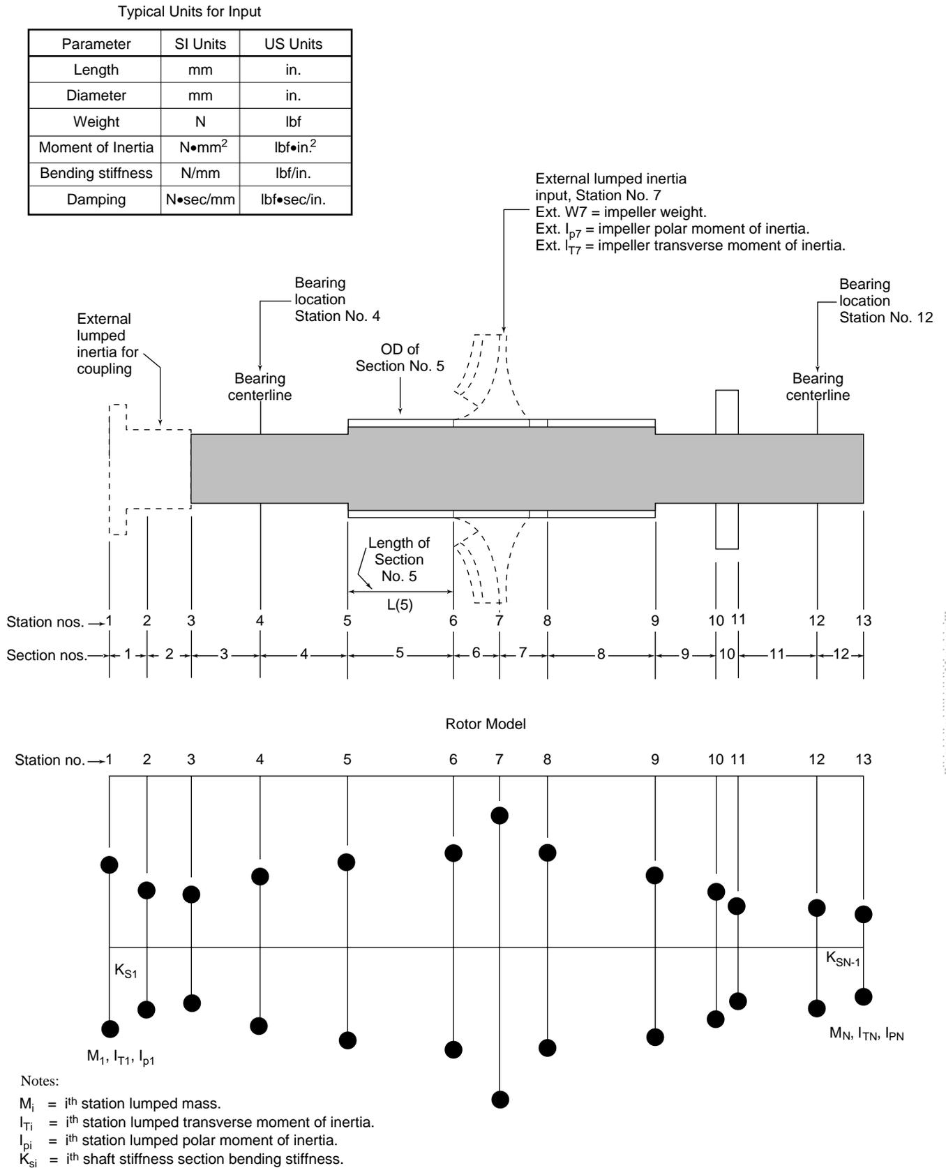
Figure 1-14—Schematic of a Lumped Parameter Rotor Model
