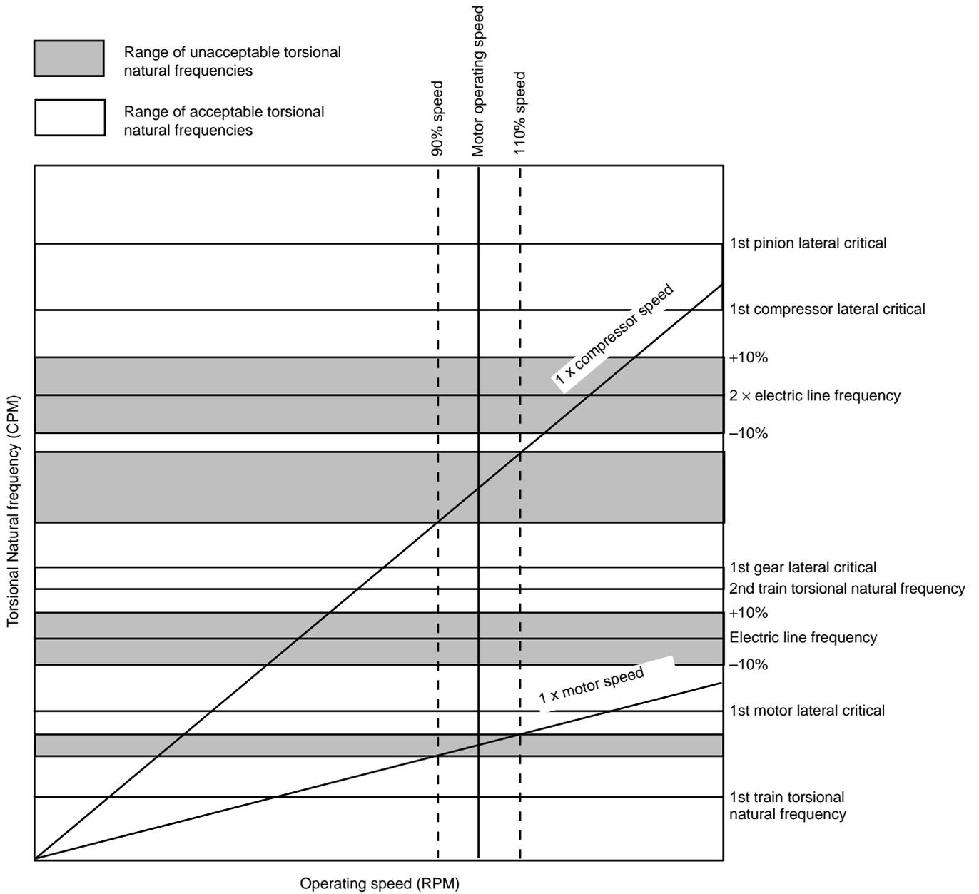
Figure 2-17—Sample Train Campbell Diagram for a Typical Motor-Gear-Compressor Train
