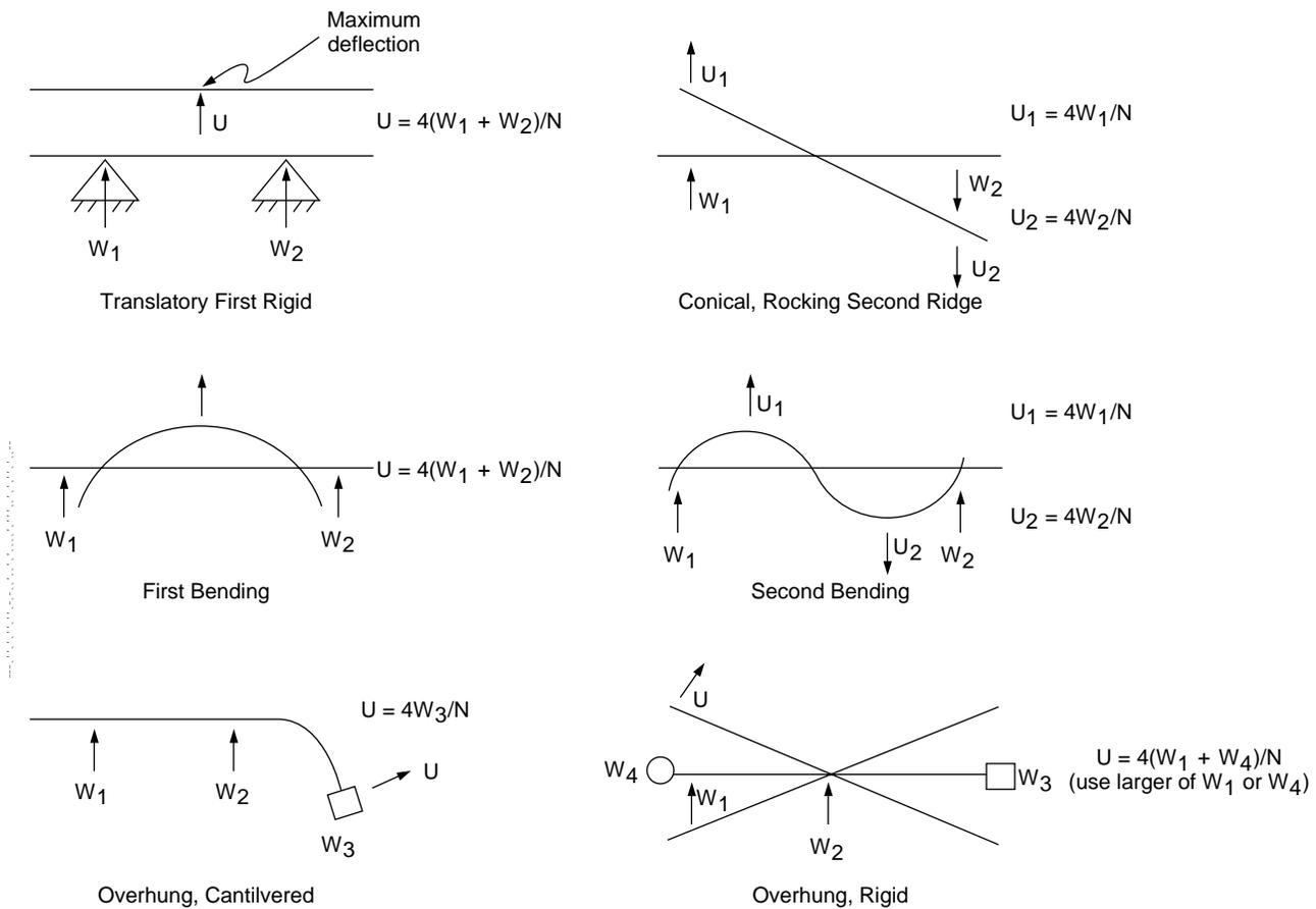
Figure 1-44—Unbalance Calculations and Placements in Figure 2 of API *Standard Paragraphs*
