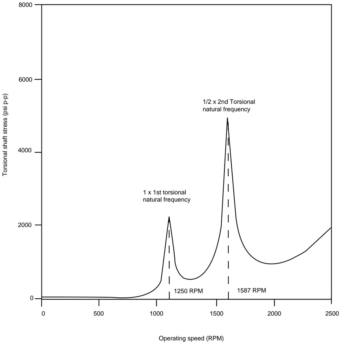
Figure 2-24—A Typical Plot of Calculated Oscillatory Stresses Versus the Reference Frequency (Low Shaft Speed)
