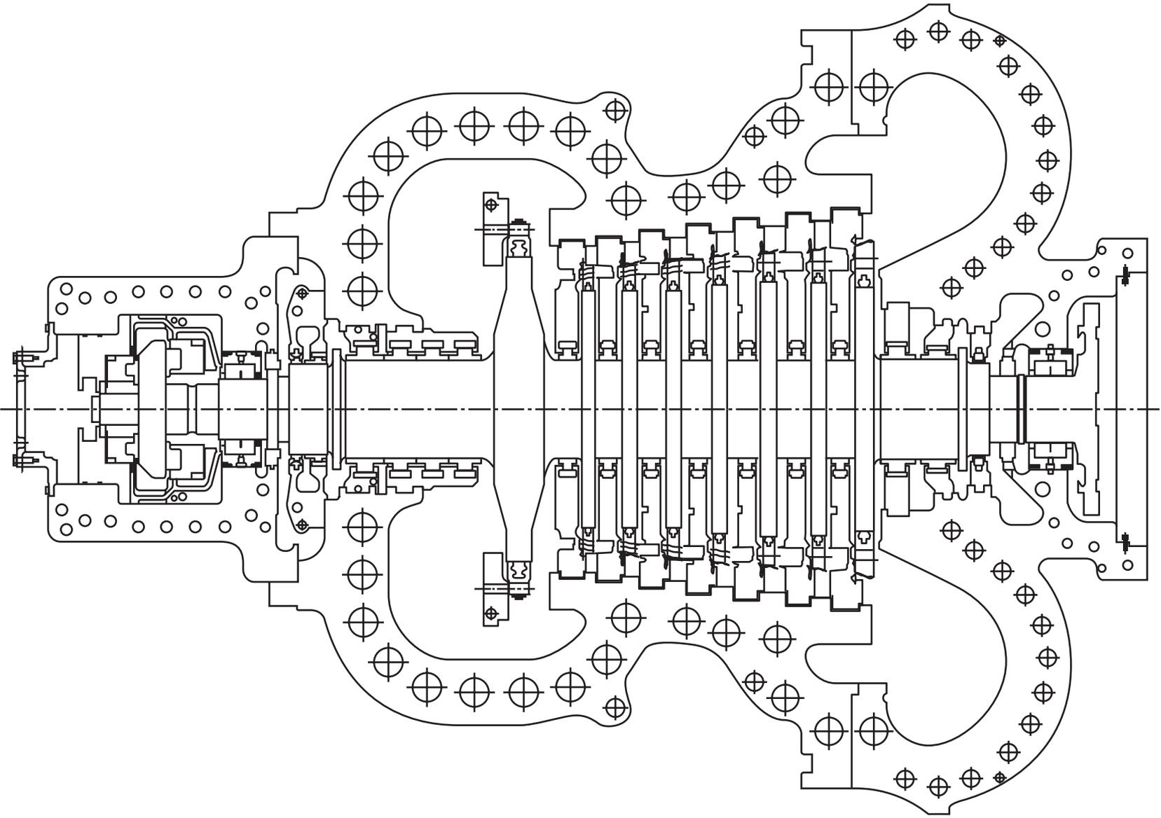
Figure 1-16—Cross Sectional View of an Eight-Stage 12 MW (16,000 HP) Steam Turbine
