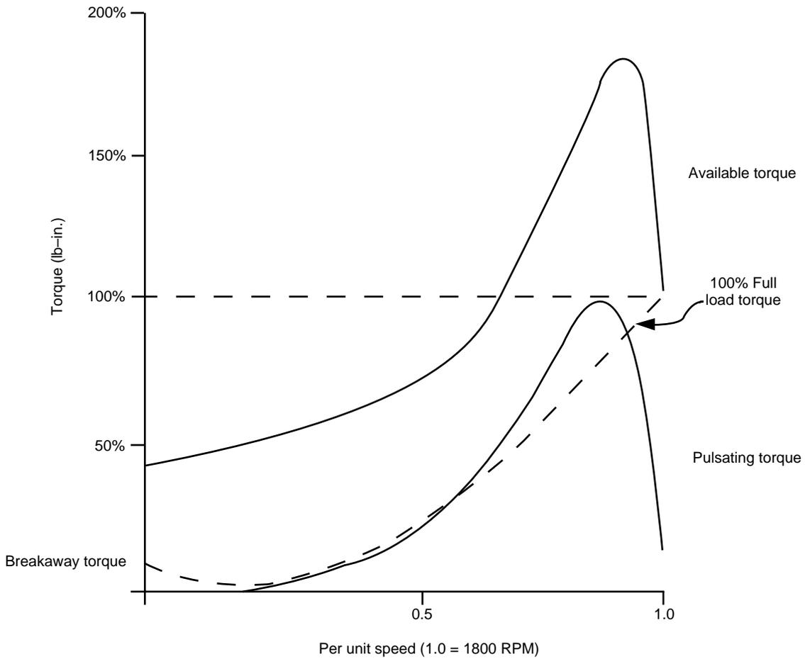
Figure 2-26—Torque Characteristics of a Typical Laminated Pole Synchronous Motor-Gear-Compressor Train
