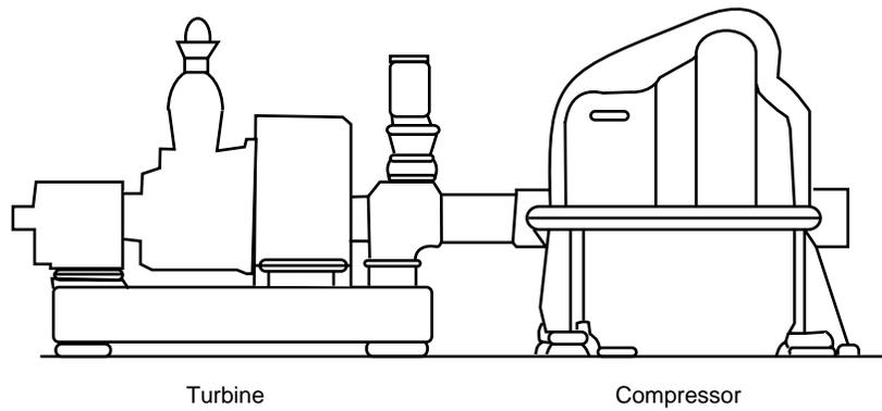
Figure 2-6—Side View of a Typical Turbine-Compressor Train
