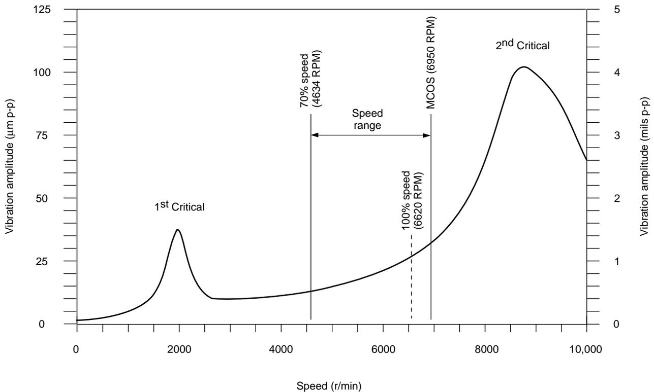
Figure 1-43—Response of a Variable Speed Steam Turbine
