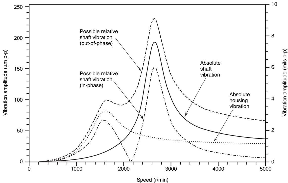
Figure 1-48—Example of Absolute Versus Relative Shaft Vibration For a Flexibly Supported Rotor Bearing System
