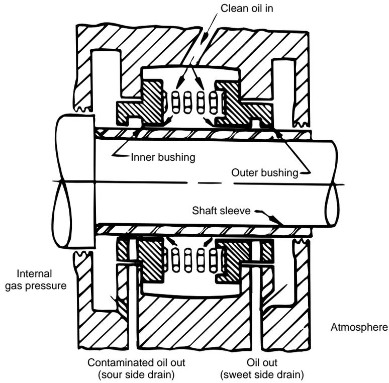
Figure 1-30—Liquid-Film Shaft Seal With Cylindrical Bushing
