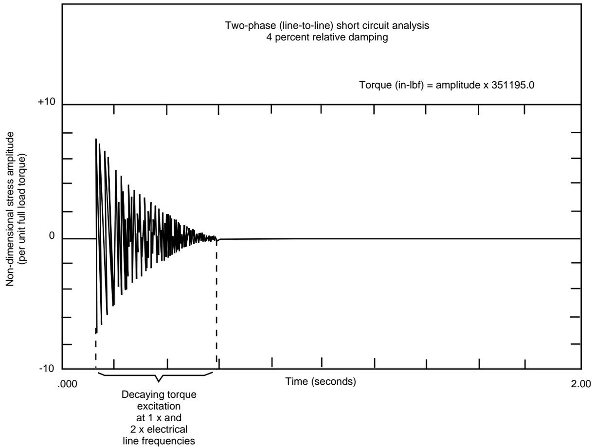
Figure 2-29—Transient Torsional Fault Analysis Worst Case Transient Fault Condition
