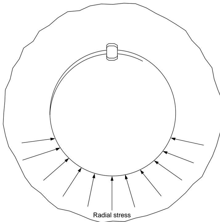
Figure 3-4—Effect of Single Key on Wheel Stiffness
