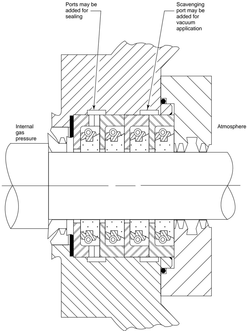
Figure 1-29—Restrictive-Ring Shaft Seal
