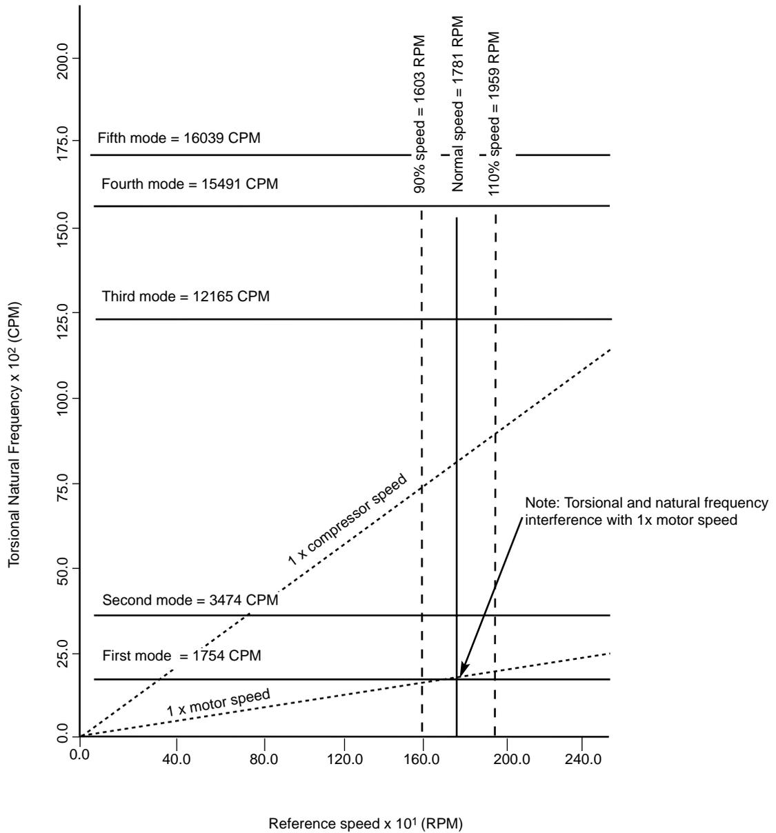
Figure 2-20—Sample Train Torsional Campbell Diagram for a Typical Motor-Gear-Compressor Train (With Unacceptable Torsional Natural Frequency Separation Margins)
