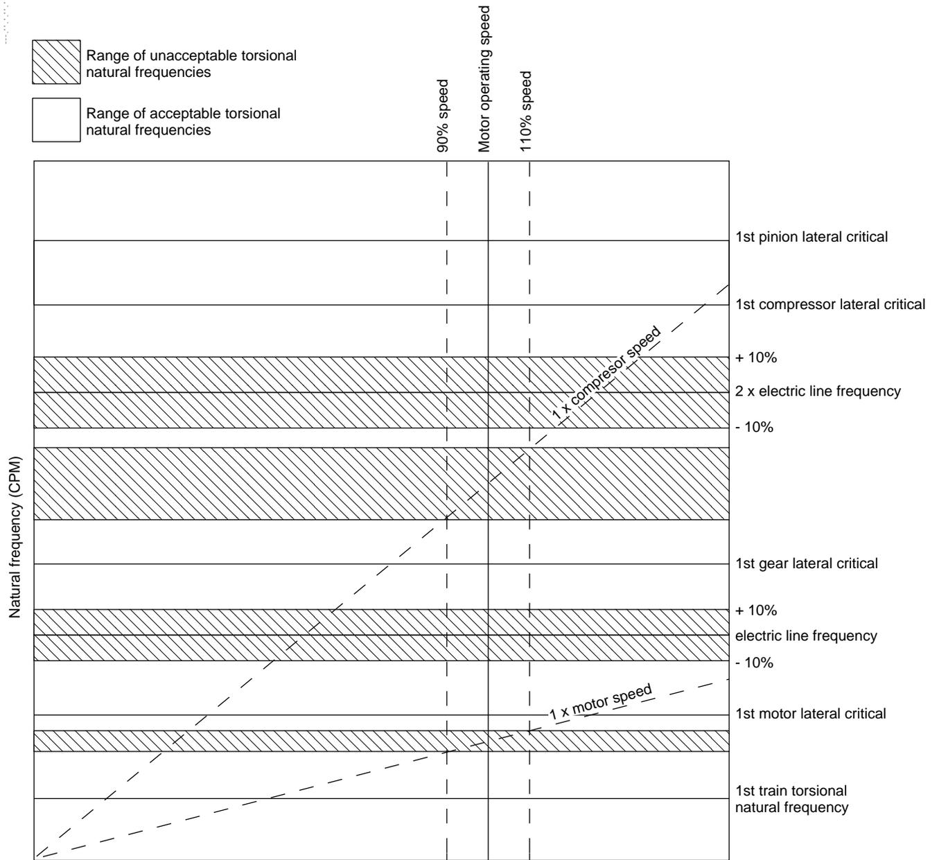
Figure 1-3—Sample Train Campbell Diagram for a Typical Motor-Gear-Compressor Train
