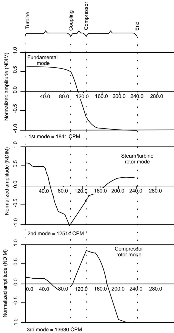
Figure 2-23—Torsional Modeshapes for a Typical Turbine-Compressor Train
