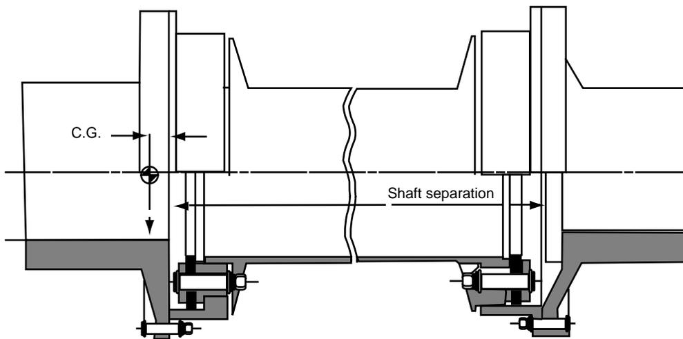
Figure 2-12—Cross-Sectional Views of Gear and Flexible Element (Disk-Type) Couplings
