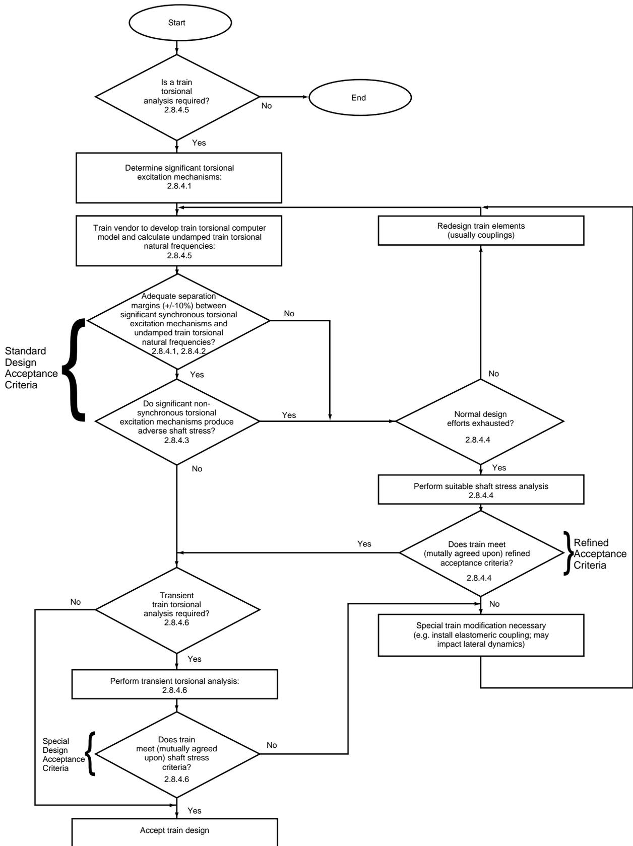
Figure 2-2—Rotor Dynamics Logic Diagram (Torsional Analysis)
