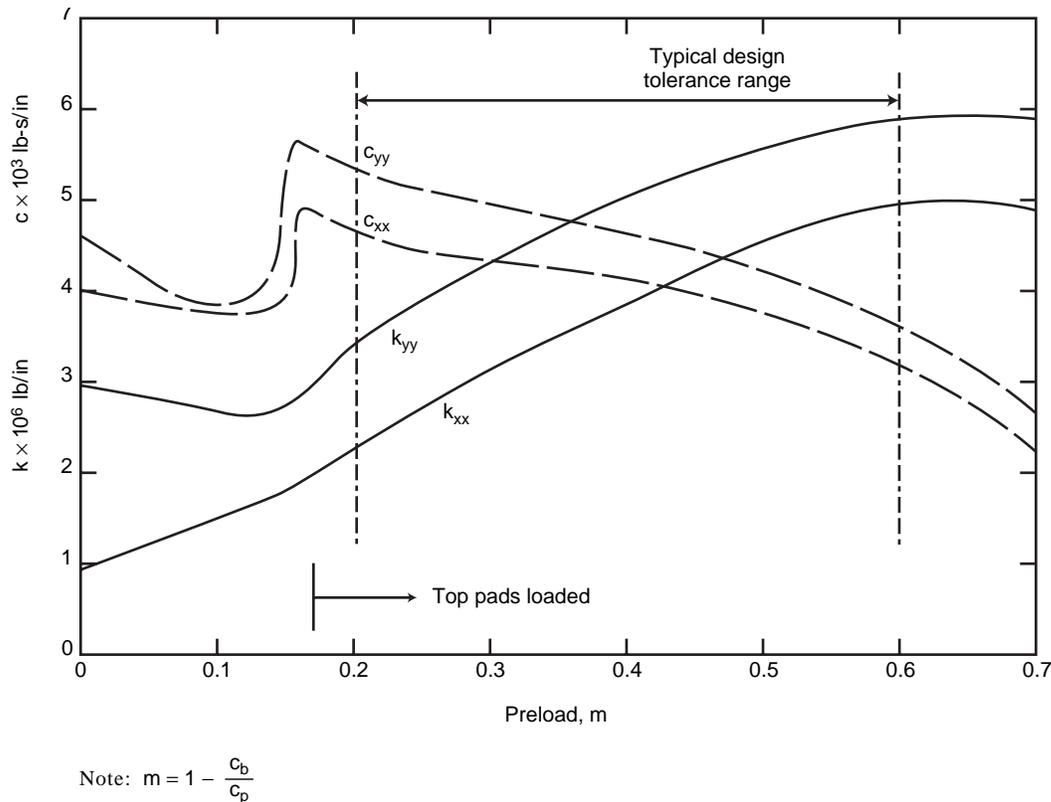
Figure 1-22—Effect of Preload on Tilting Pad Bearing Coefficients
