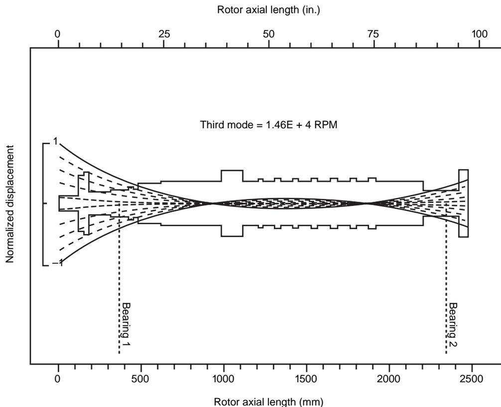
Figure 1-37—Third Mode Shape for Eight-Stage Steam Turbine
