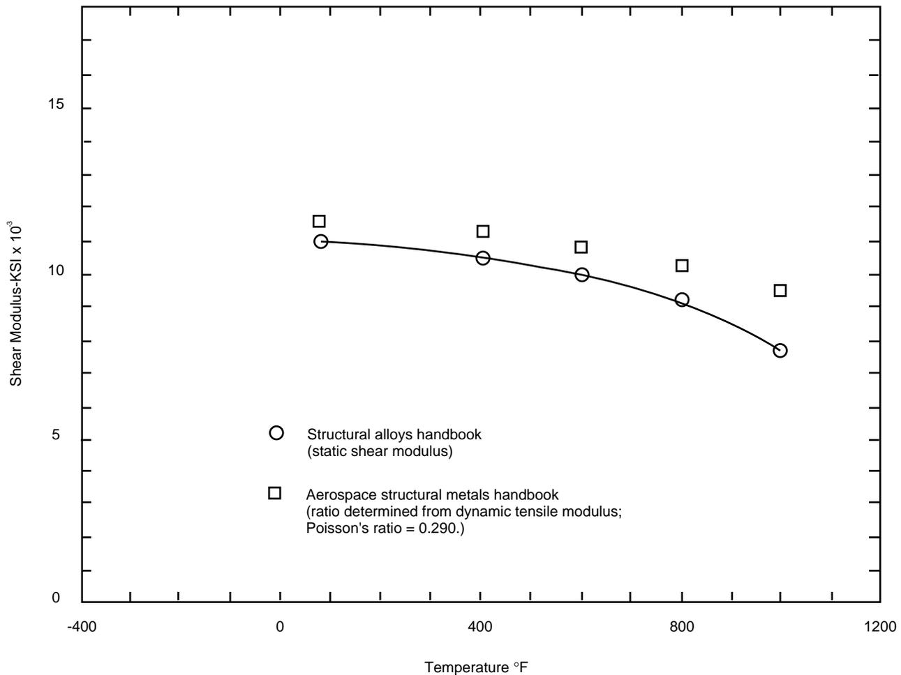
Figure 2-16— Variation of Shear Modulus With Temperature
