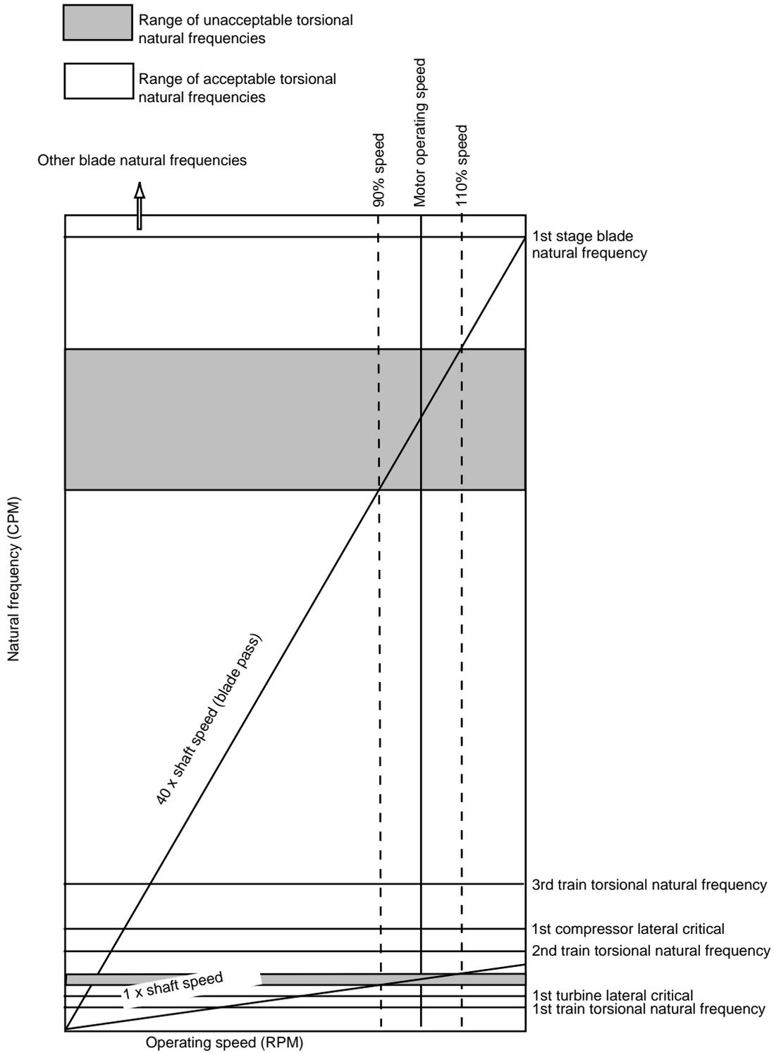
Figure 2-18—Sample Train Campbell Diagram for a Typical Turbine-Compressor Train
