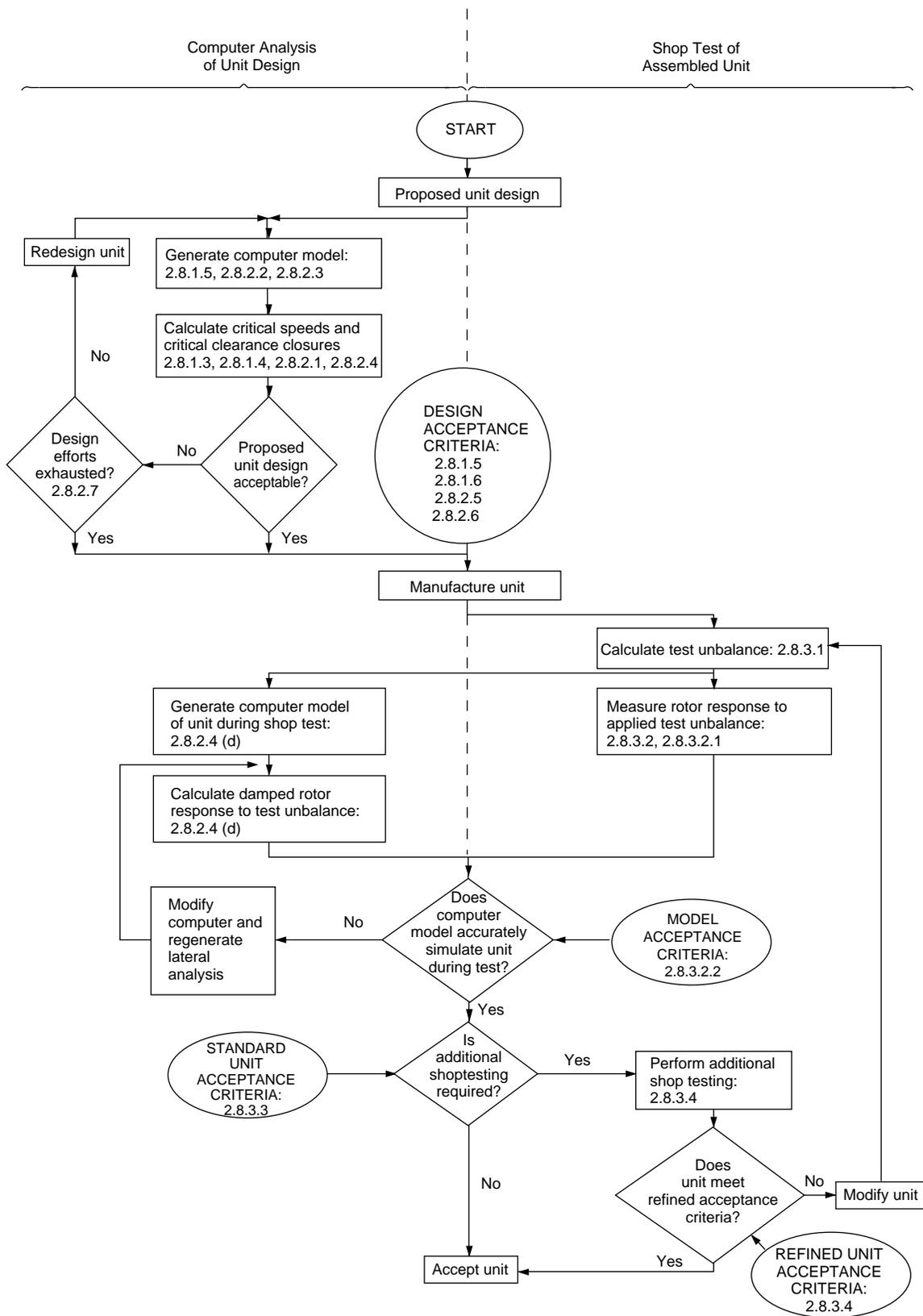
Figure 1-34—Detailed Flow Chart of API Vibration Acceptance Program Outlined in API *Standard Paragraphs*
