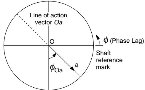
Step 2. Apply the trial unbalance,  $U_{\text{trial}}$ , and measure the resulting vibration vector,  $Ob$ , at the operating speed nearest the critical speed of concern. Vibration vector  $Ob$  is generated by the residual plus the trial unbalances.
