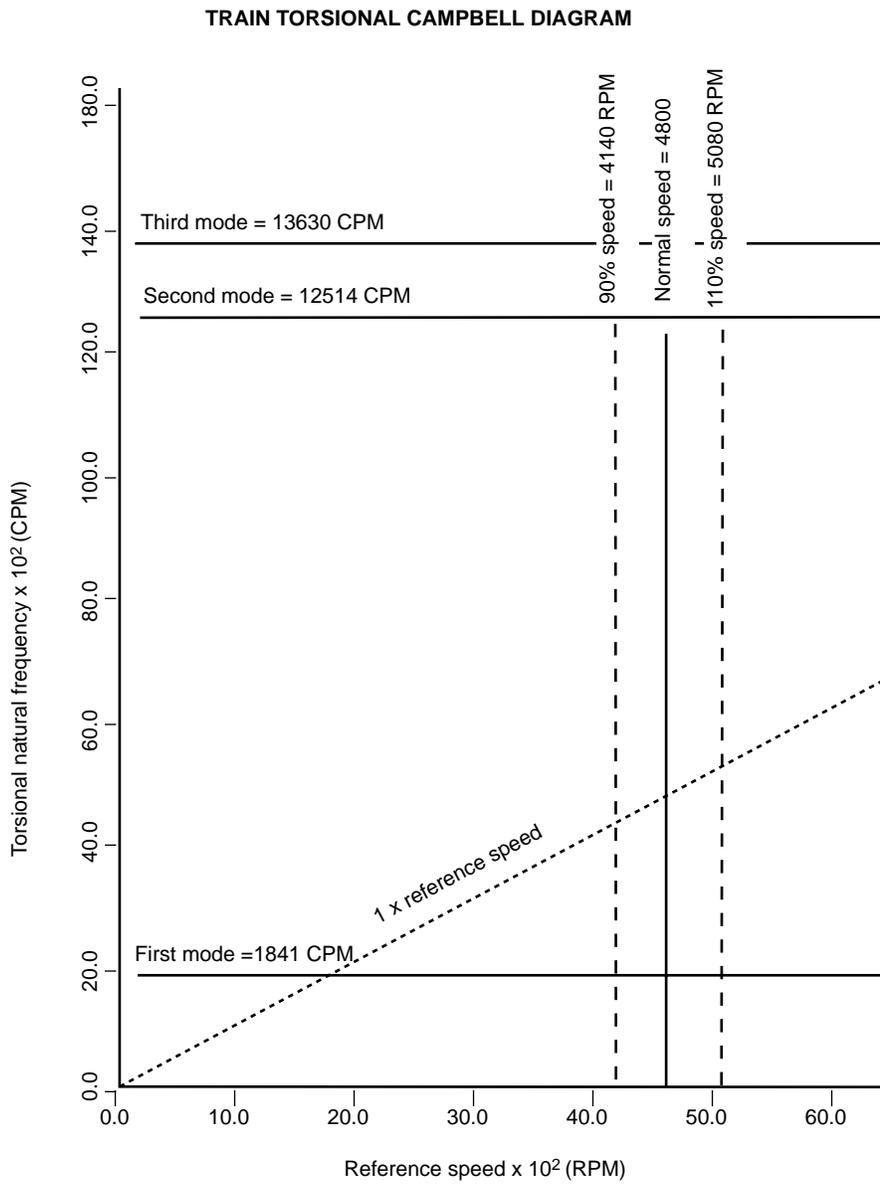
Figure 2-22—Sample Train Torsional Campbell Diagram for a Typical Turbine-Compressor Train
