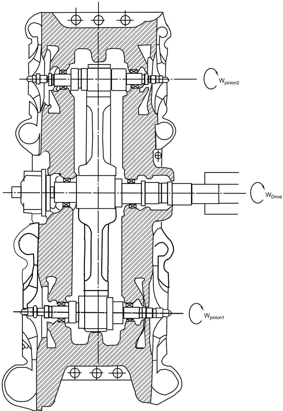
Figure 2-9—Multi-Speed Integrally Geared Plant Air Compressor
