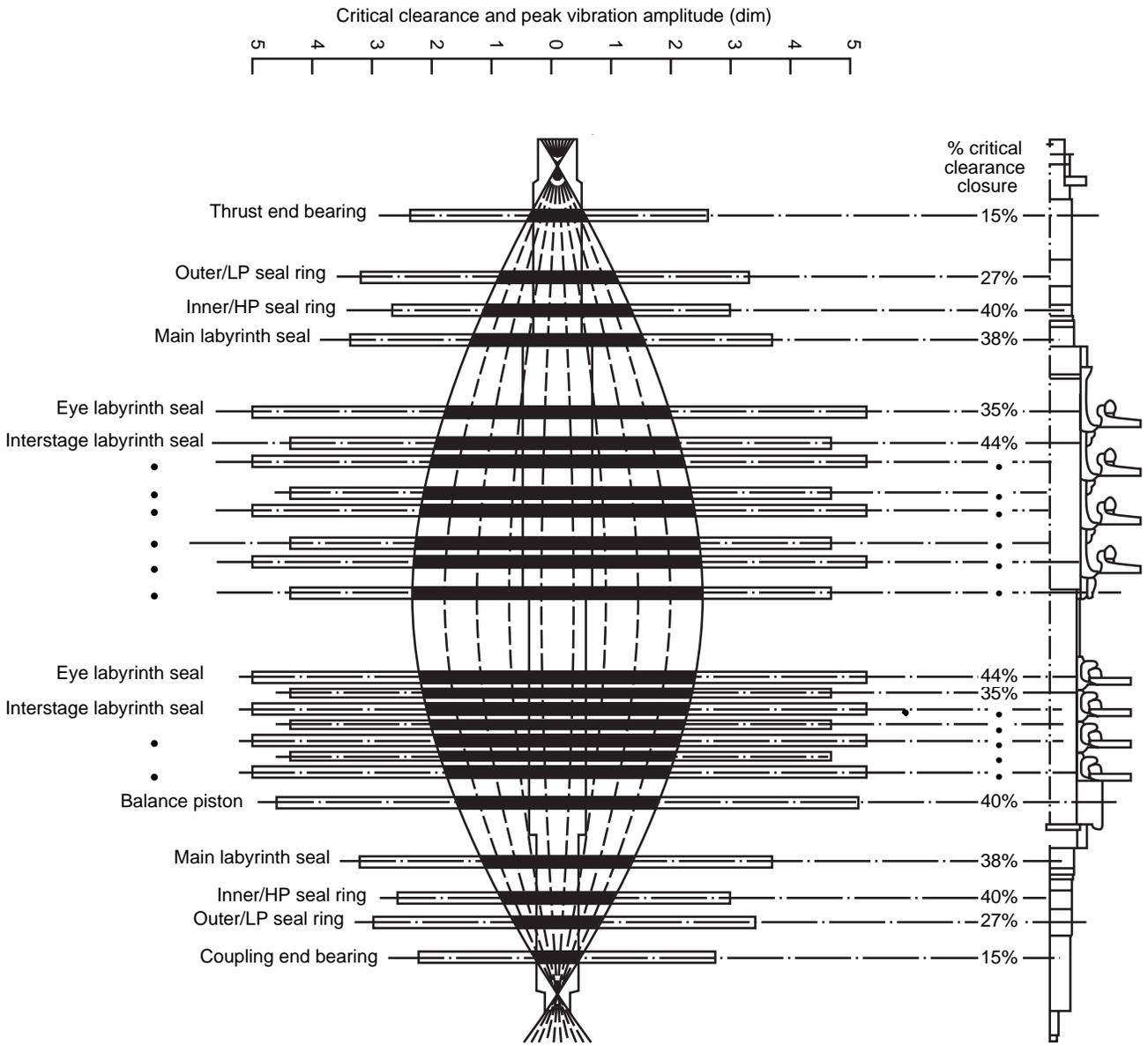
Figure 1-45—Modal Diagram Showing Critical Clearances and Peak Vibration Levels
