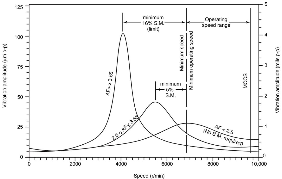
Figure 1-49—API Required Separation Margins for Operation Above a Critical Speed
