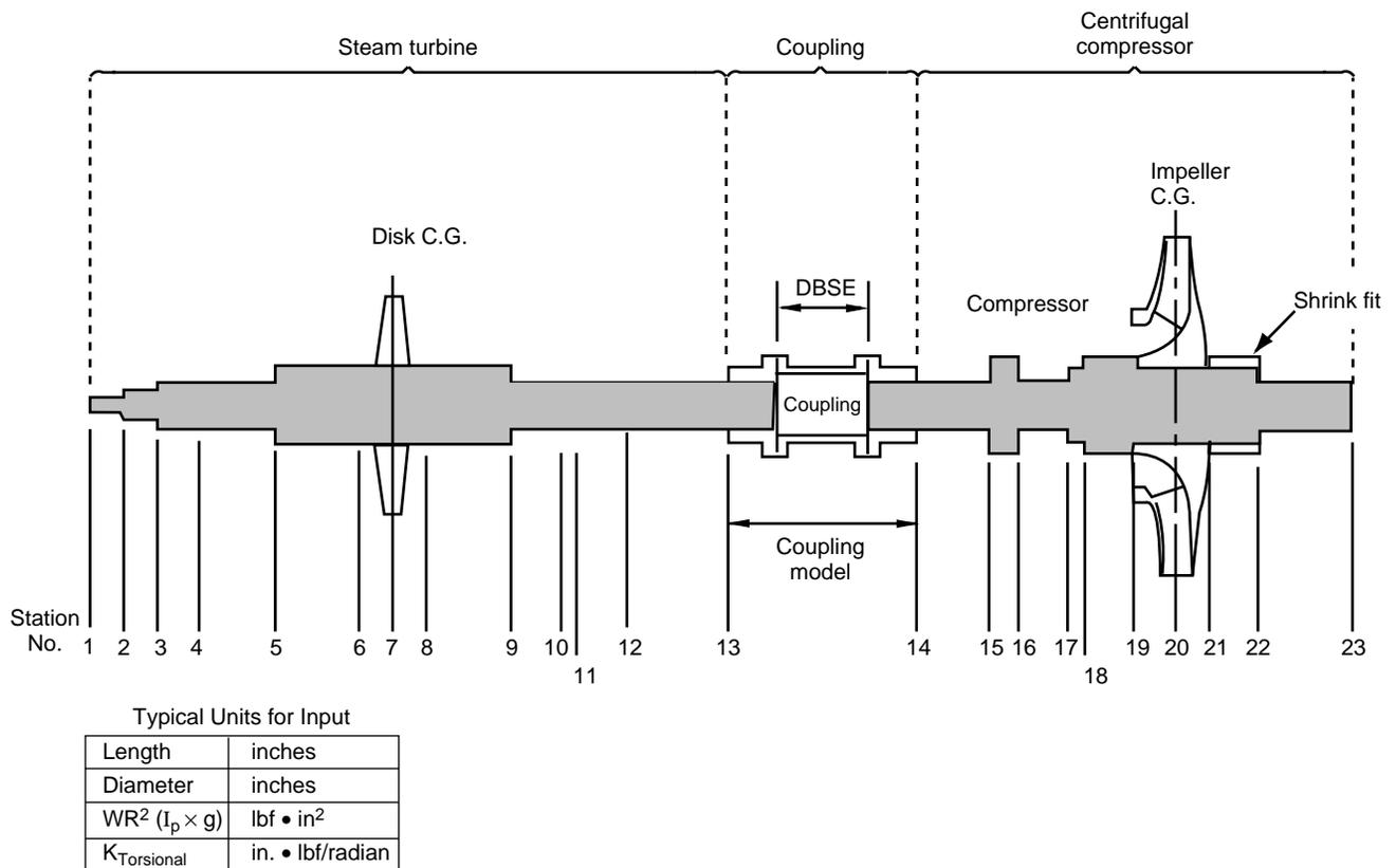
Note: Coupling vendors typically provide  $WR^2$  and  $K_{Torsional}$  for each coupling. The  $WR^2$  value does not included the  $WR^2$  of the coupling journal (shaft inside the coupling HUB). The  $K_{Torsional}$  value typically assumes  $1/3$  shaft penetration into the coupling HUB.
