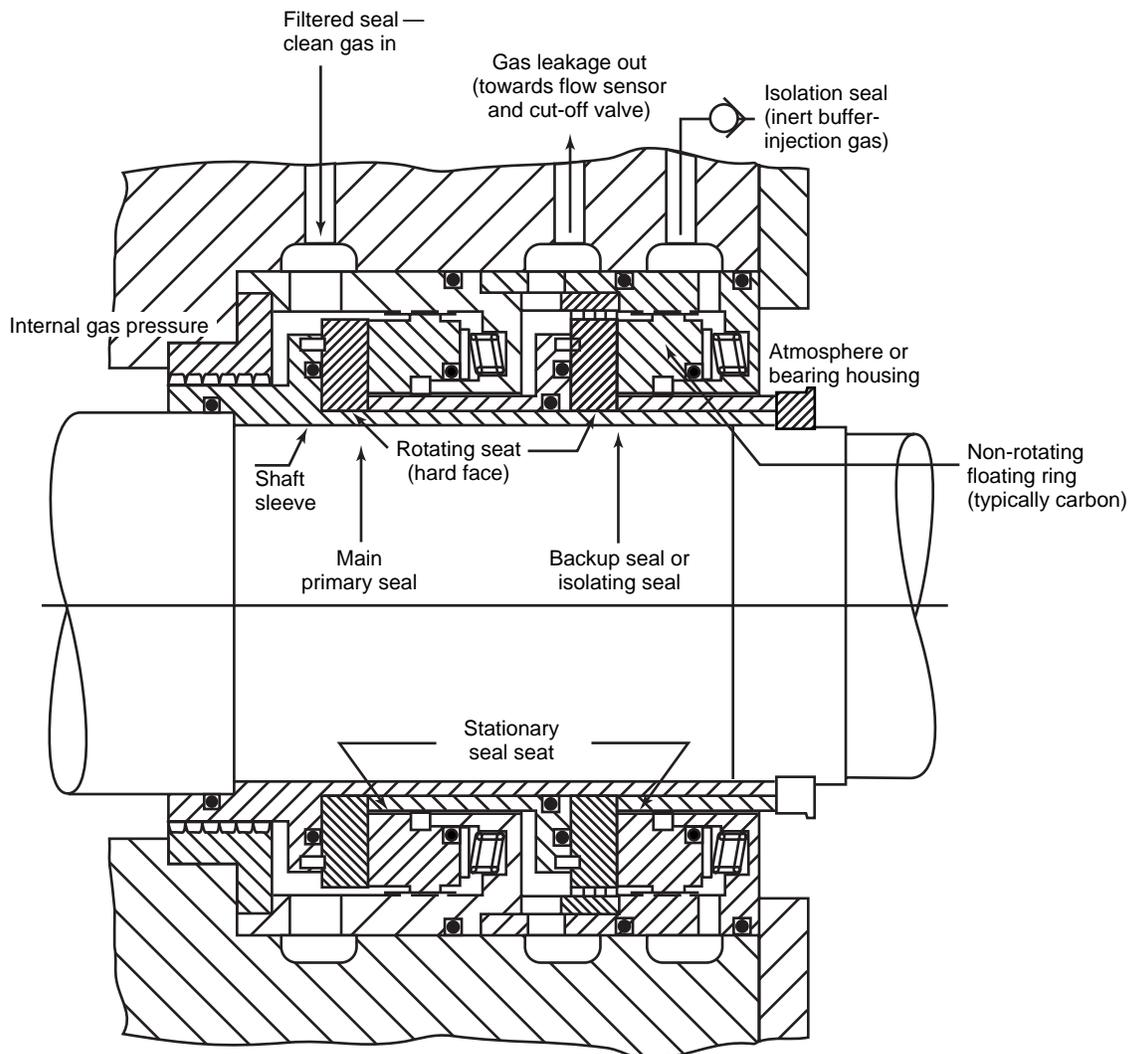
Figure 1-32—Self-Acting Gas Seal
