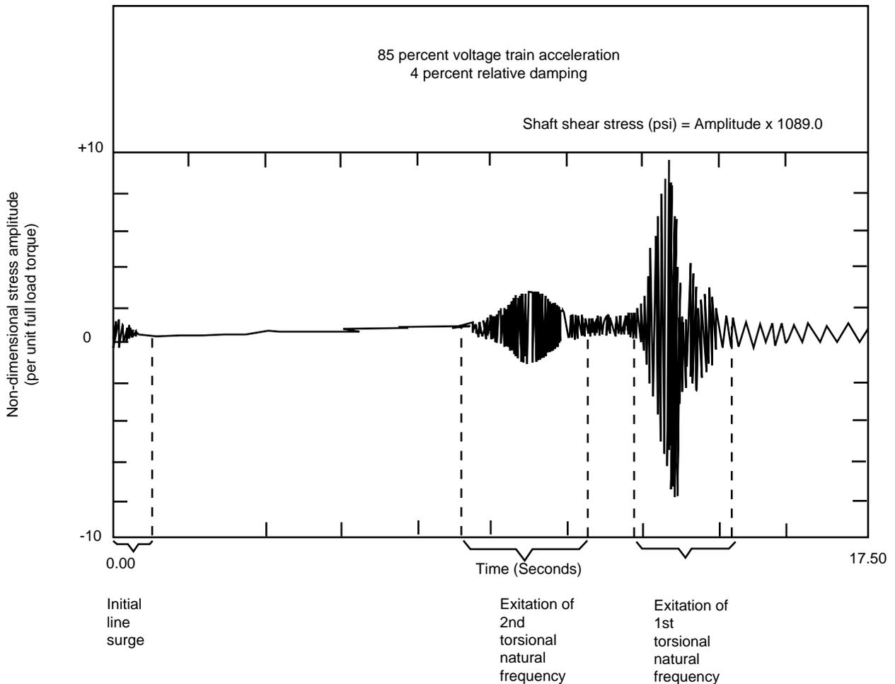
Figure 2-25—Transient Torsional Start-Up Analysis Maximum Stress Between Gear and Compressor
