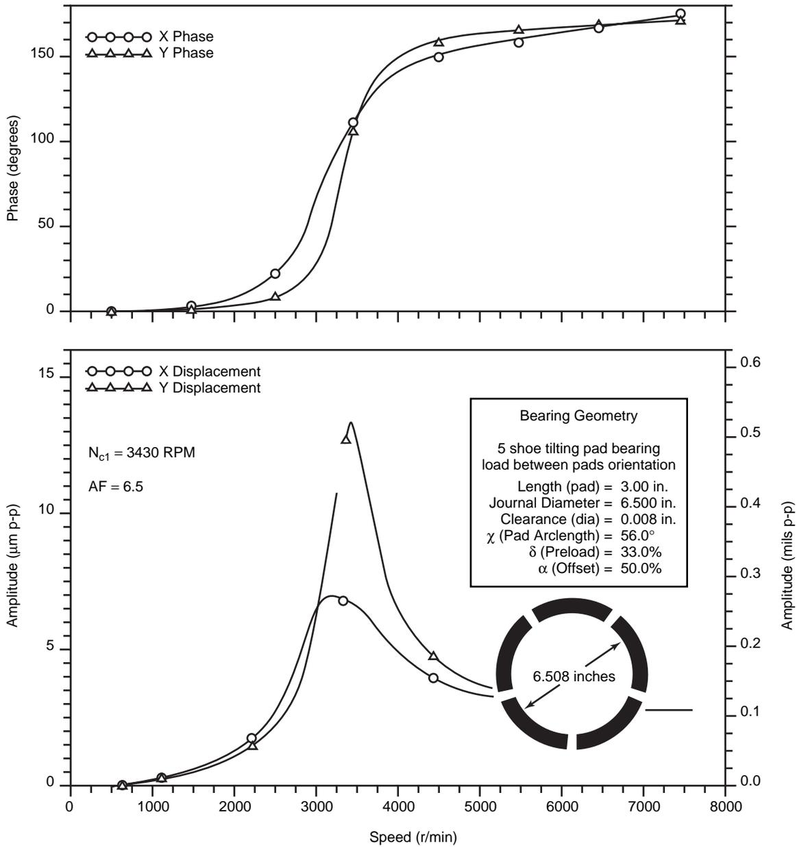
Figure 1-2—A Sample Bode Plot: Calculated Damped Unbalance and Phase Responses of an Eight-Stage 12 MW(16,000 HP) Steam Turbine
