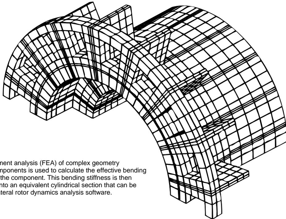
A finite element analysis (FEA) of complex geometry rotating components is used to calculate the effective bending stiffness of the component. This bending stiffness is then converted into an equivalent cylindrical section that can be input into lateral rotor dynamics analysis software.
