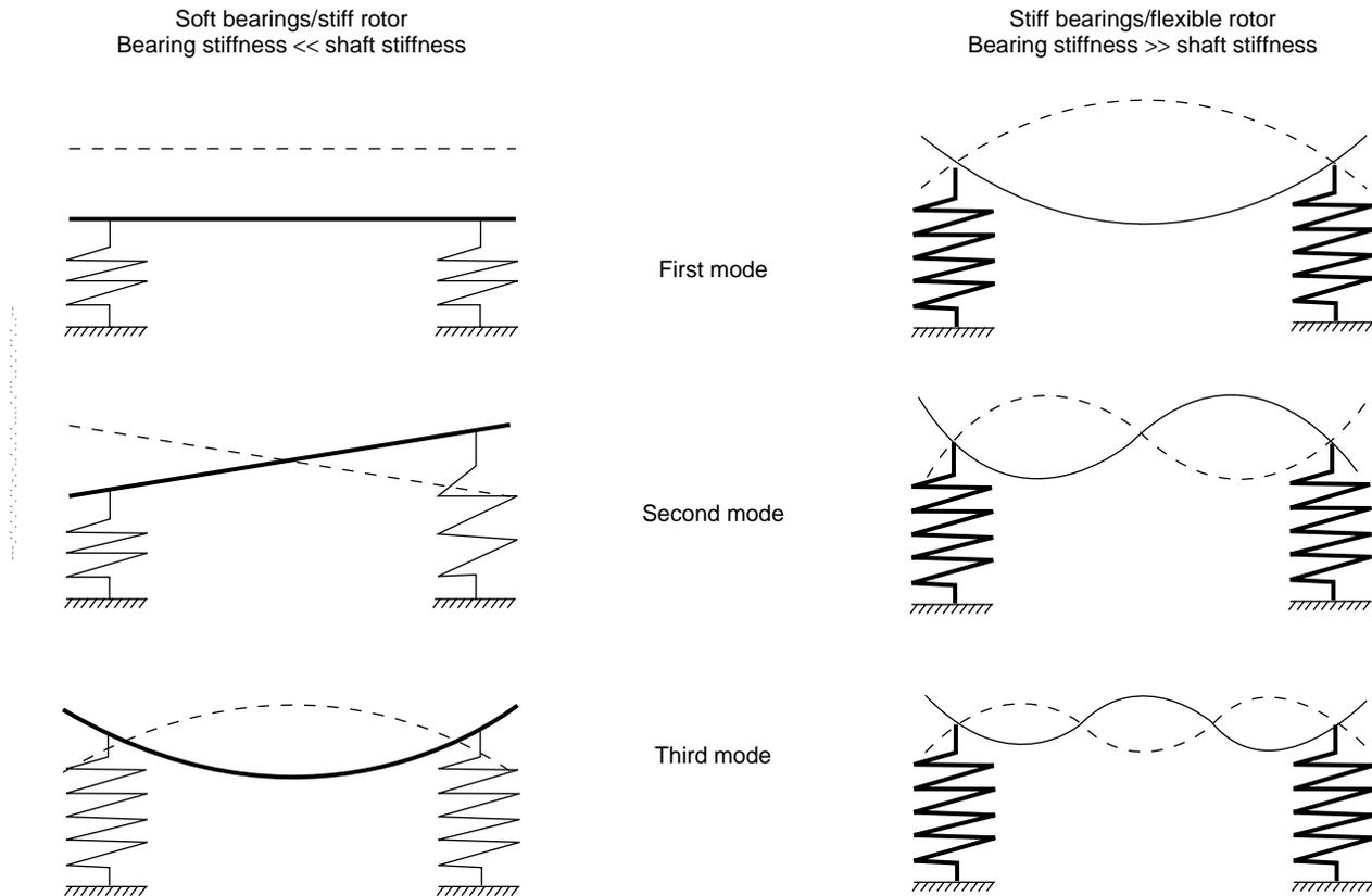
Figure 1-6—Mode Shape Examples for Soft and Stiff Bearings
