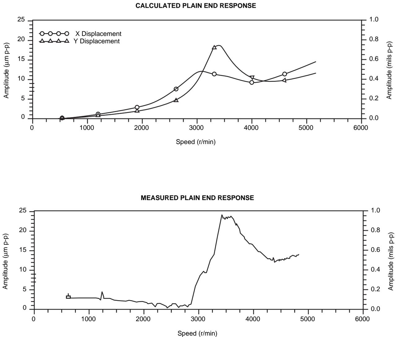
Figure 1-41—Comparison of Calculated and Measured Unbalanced Responses
