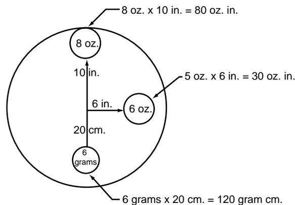
Figure 3-1—Units of Unbalance Expressed as the Product of the Unbalance Weight and its Distance From the Center of Rotation
