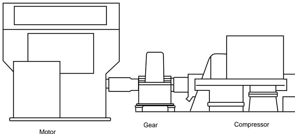
Figure 2-3—Side View of a Typical Motor-Gear-Compressor Train
