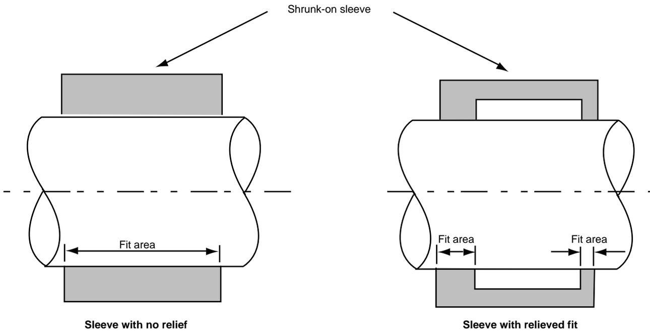
Figure 2-11— Examples of Shrunk-On Shaft Sleeves With and Without Relieved Fits
