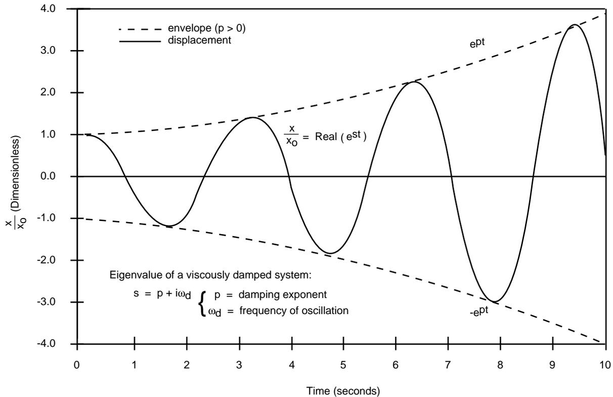
Figure 1-13—Motion of an Unstable System Undergoing Free Oscillations
