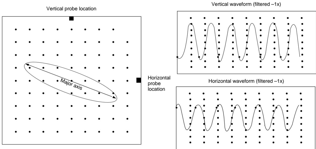
Figure 1-51—Determination of Major Axis Amplitude From a Lissajous Pattern (Orbit) on an Oscilloscope
