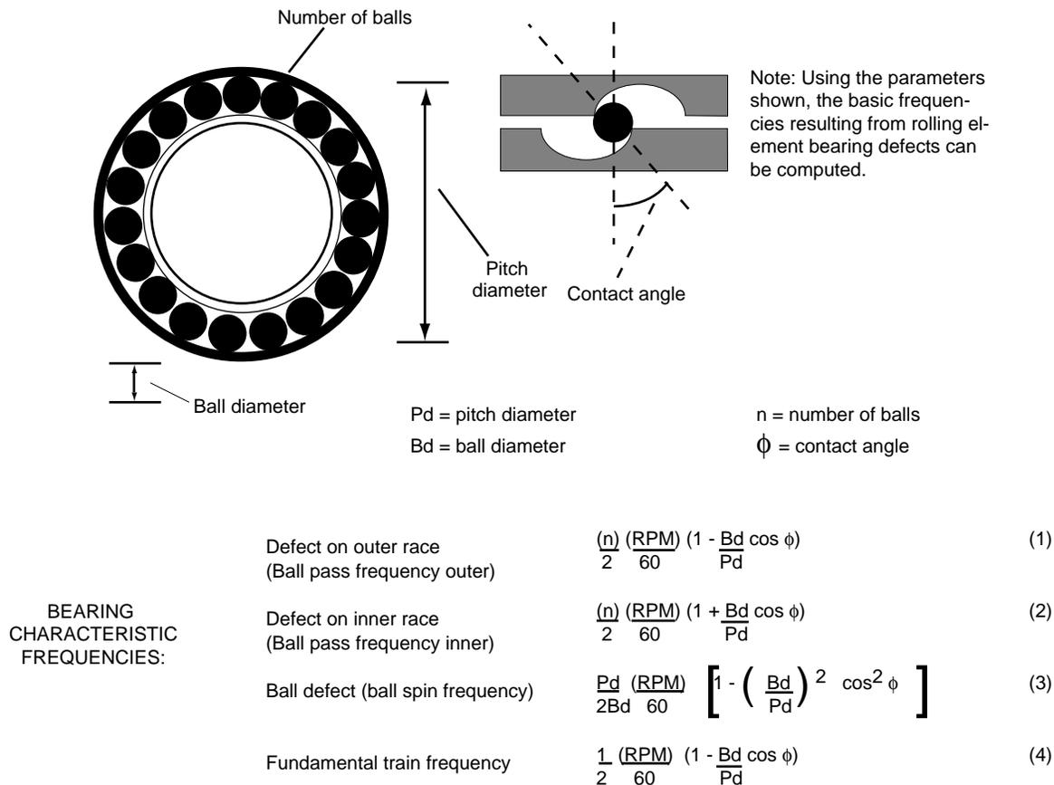
Figure 1-39—Anti-Friction Bearing Design Characteristics
