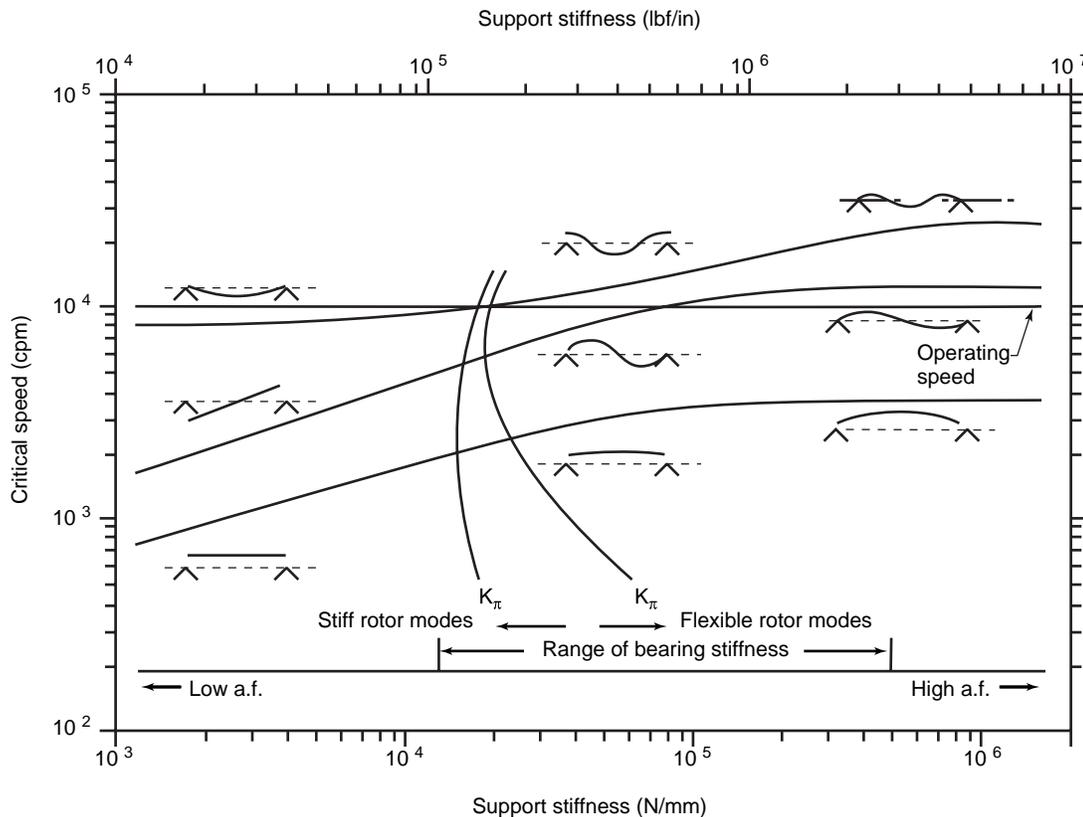
Figure 1-5—Undamped Critical Speed Map
