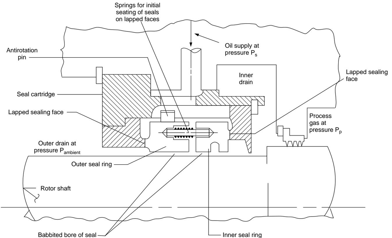
Figure 1-23—Oil Bushing Breakdown Seal
