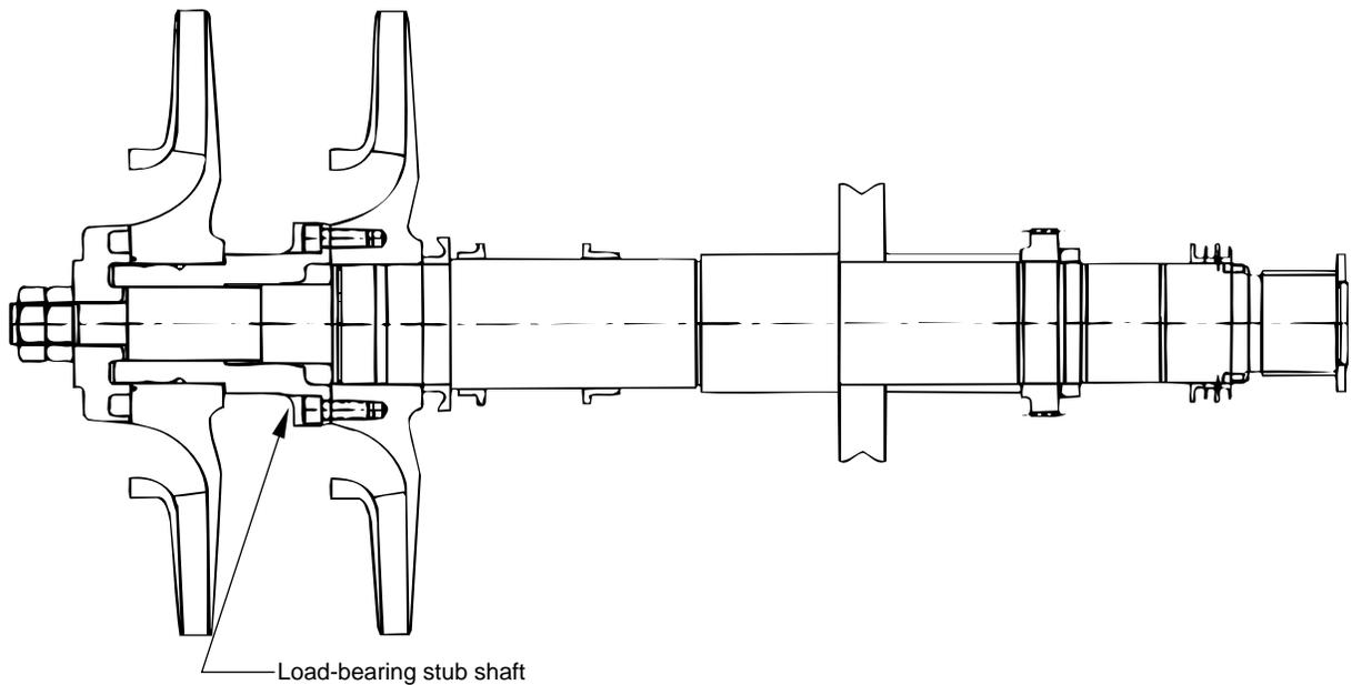
**Cross-Section of Rotating Element
